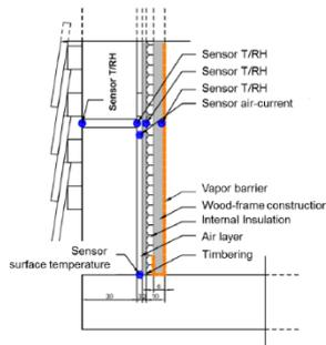
Proposed sensors network allow to collect data of all the relevant parameters and metrics for characterizing the energy behaviour of the building, the climate situation and comfort in the rooms, the climate-related stress on valuable surfaces, moisture and heat situation in the energy upgraded building construction and energy consumption.
