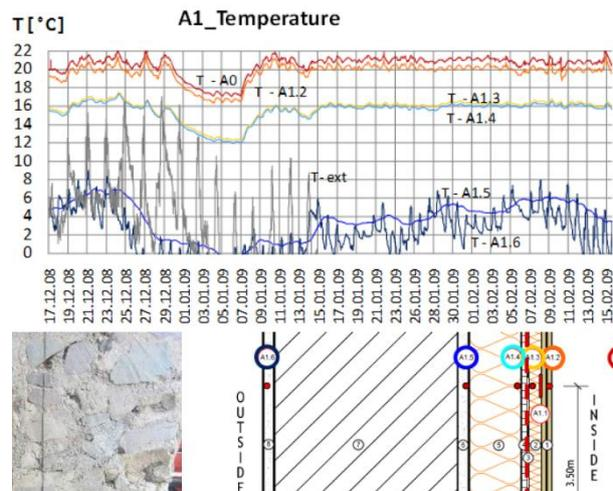
However, in Bolzano cooling demand rises with more insulation, since the low night temperature would allow for some heat rejection through wall during night. Nevertheless, the absolute savings in cooling energy without insulation are small compared to the additional heat losses in winter without insulation – the all year optimisation is still clearly in favour of insulation!
