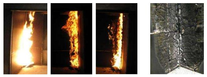
Figure 11. Uncoated furan-flax (cork core) sandwich panel (right: damaged surface after end of test)
