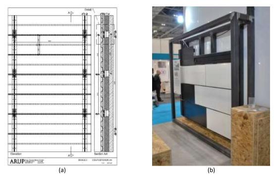
Figure 8. Detailed drawings (a) for the External Cladding Kit and its final appearance (b).
