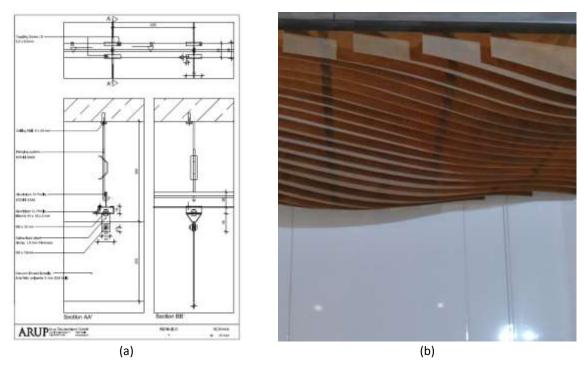
Figure 10. Detailed drawings (a) for the Suspended Ceiling Kit and its final appearance (b).
