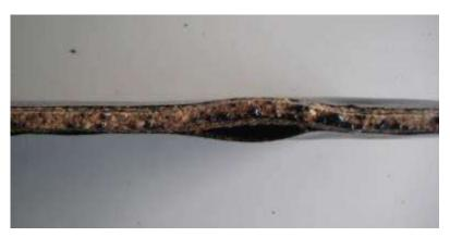
Figure 4. Result of a preliminary feasibility trial showing the effect of uncontrolled steam production during the cure of polyfurfuryl alcohol laminates with a cork core.
