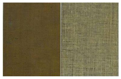
Figure 3. Jute-biopolyester sample as moulded (left) and after 12w accelerated weathering (right) to illustrate the need for a weather resistant coating on the biocomposites.
