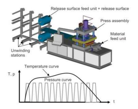
Figure 6. The semi-continuous compression moulding process
