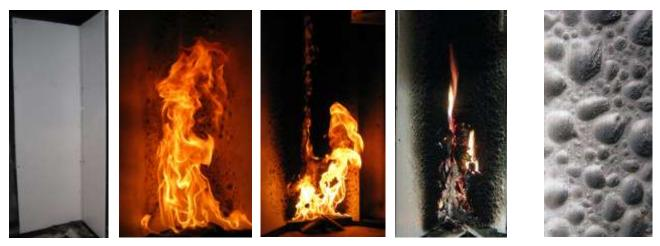
Figure 12. Furan-flax sandwich panel (as in Figure 11) coated with intumescent coating system (left) subjected to an SBI test (centre) showing surface intumescence after end of test (right).
