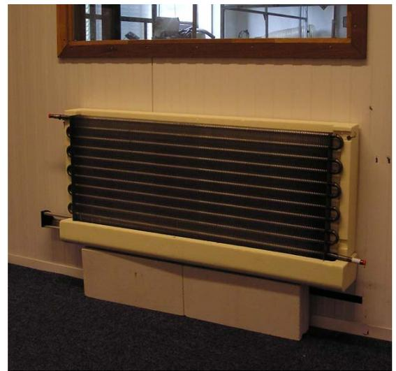
11. Prototype with heat exchanger
