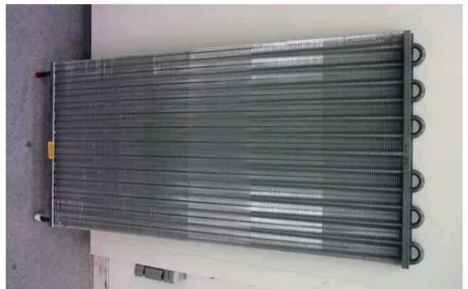
4. Principle of a single coil finned heat exchanger; 5. Tested heat exchanger.
