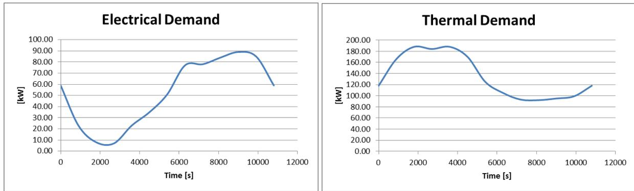
Figure 26: Conflicting profiles: low electrical demand and high thermal demand in the first half of the test and vice versa in the second half.
