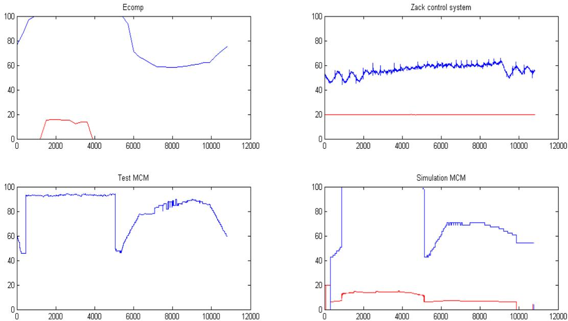
Figure 28: Results of the 4 runs **with** storage: *blue* line: output power of the *mGT*, *red* line: output power of the *ICE*
