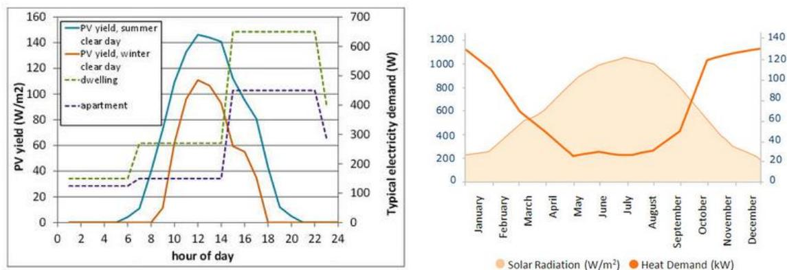
Figure 1: Mismatch between supply of renewable electricity from Photo Voltaic panels and electricity demand (left) and mismatch between supply of renewable heat from solar thermal panels and heat demand
