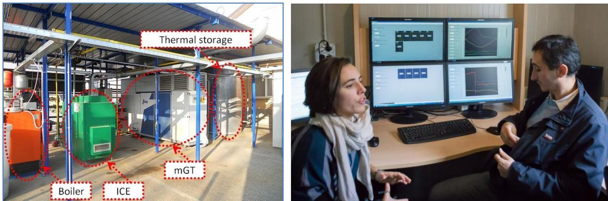
*Figure 25: Left: equipment at the lab at TPG-DIME, with a boiler, an Internal Combustion Engine CHP (ICE), a micro gasturbine CHP (mGT) and thermal storage vessel. Right: TPG-DIME personnel at the data acquisition and control system.*
