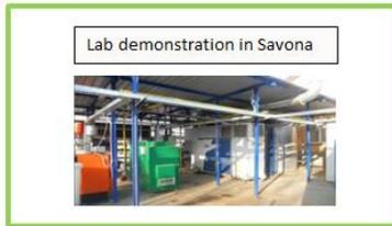
The second application of a smart energy management is the demonstration of the Multi Commodity Matcher in a real lab environment controlling the operation of several cogeneration units. This required producing an interface allowing the communication between the MCM control algorithm running in Matlab and the data acquisition and control system, running in LabVIEW. The equipment controlled included:
