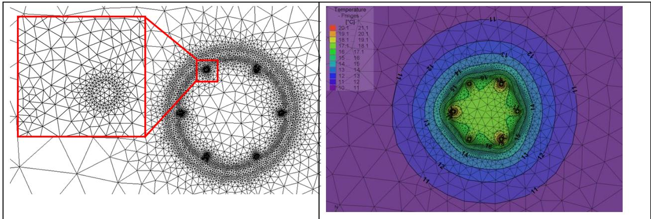
Figure 6: Calibrated high detail 3D-FEM models to analyse the performance of new materials in thermo-active foundations.
