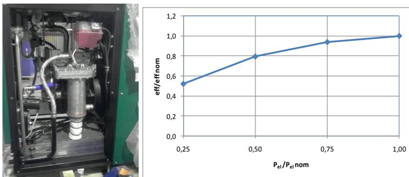
Figure 5: Picture and electrical efficiency of an internal combustion engine CHP at partial load.
