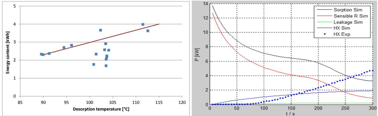
Figure 15: Energy content of the TNO 3 kWh reactor vs. desorption temperature (left) and model calculation (lines) and experimental values of thermal powers as a function of time (right) for a particular experiment.
