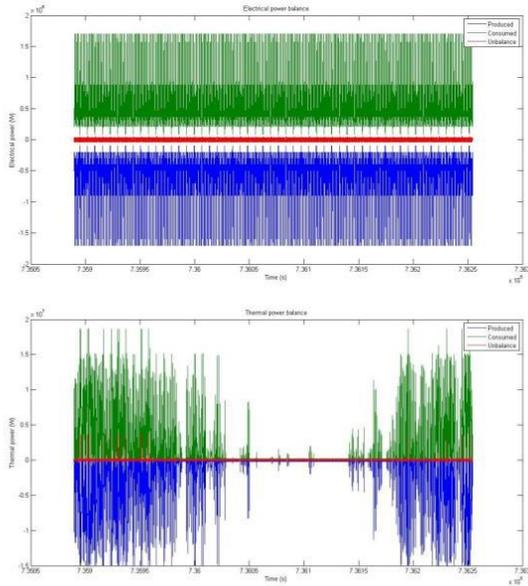
Figure 22: Electricity profile (top) and heat profile (bottom) during the whole year in the BAU scenario of Tweewaters. (blue = production, green = consumption, red = unbalance)
