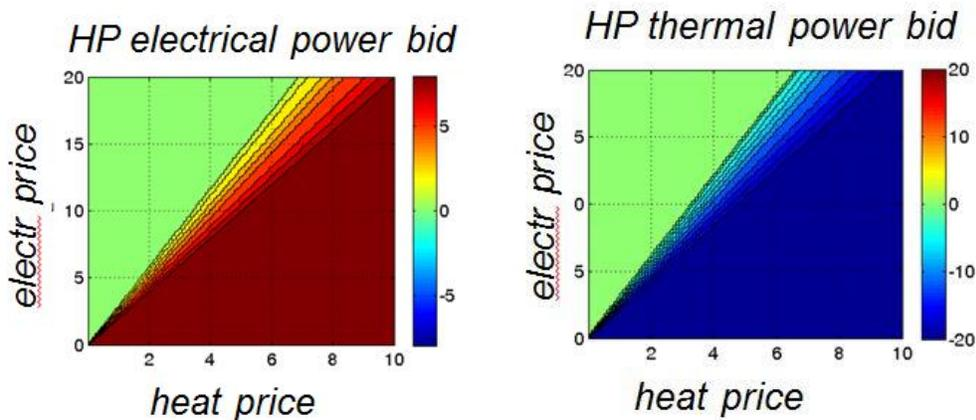
Figure 19: Electrical power bid surface (left) and thermal power bid surface (right) of a heat pump. The colours represent the amount of power the heat pump is willing to produce as a function of the prices of heat and electricity. As an example, at an electricity price of 5 €/kWh and a heat price of 6 €/kWh the heat pump will be fully on, consuming 6.7 kWh of electricity and producing 20 kWh of heat
