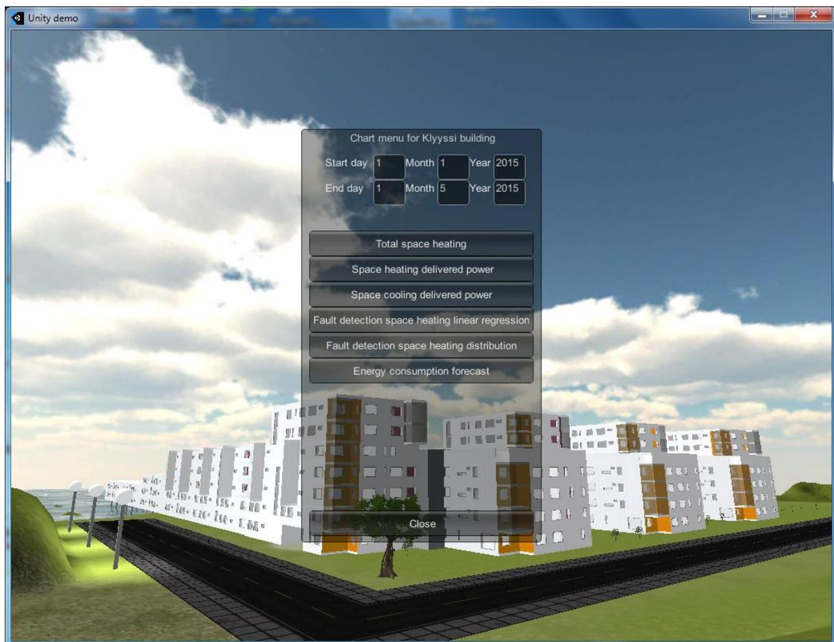
**Figure 21** Example of menu started by clicking the building in Unity game engine based 3D model.
