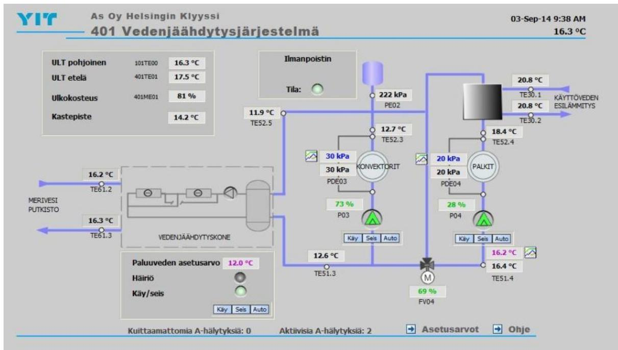
Figure 11 Cooling network process view for remote controlling
