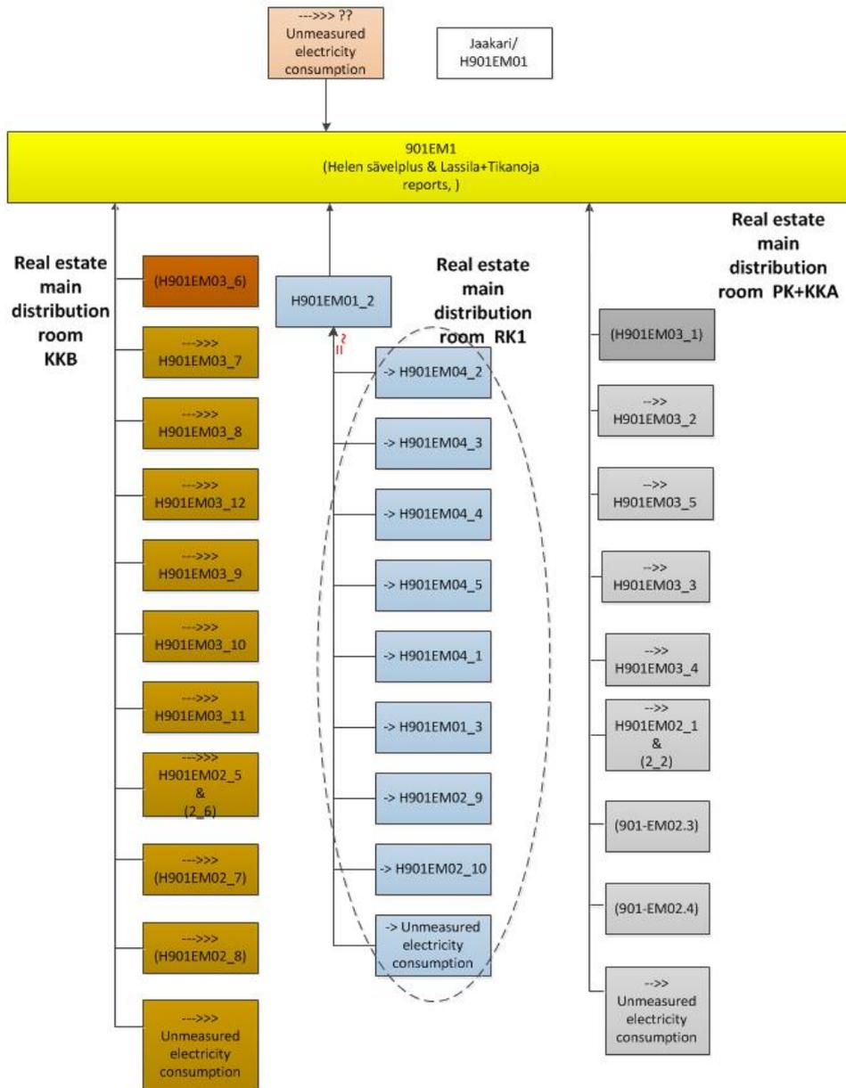
Figure 26 Hierarchical structure of electricity meters
