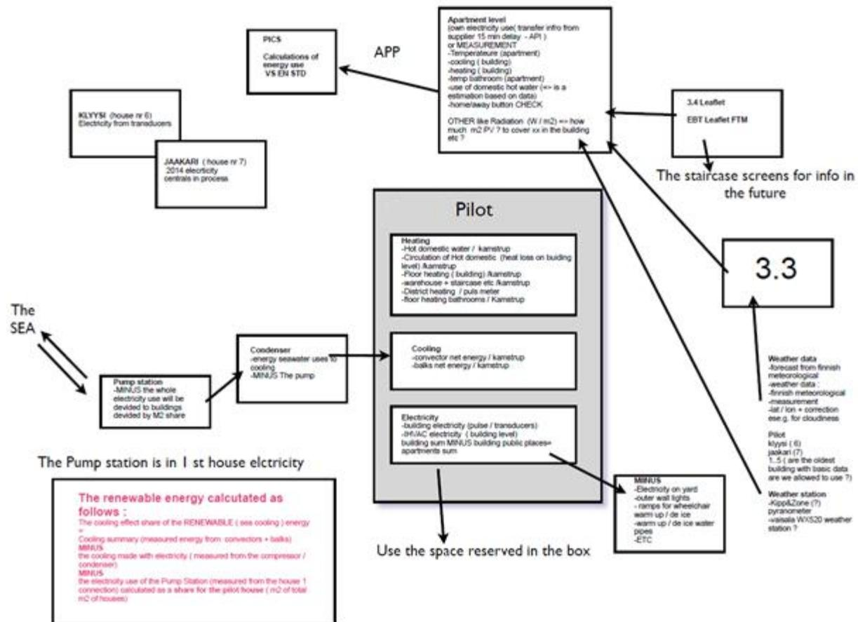
*Figure 3 Pilot software and EEPOS connections*
