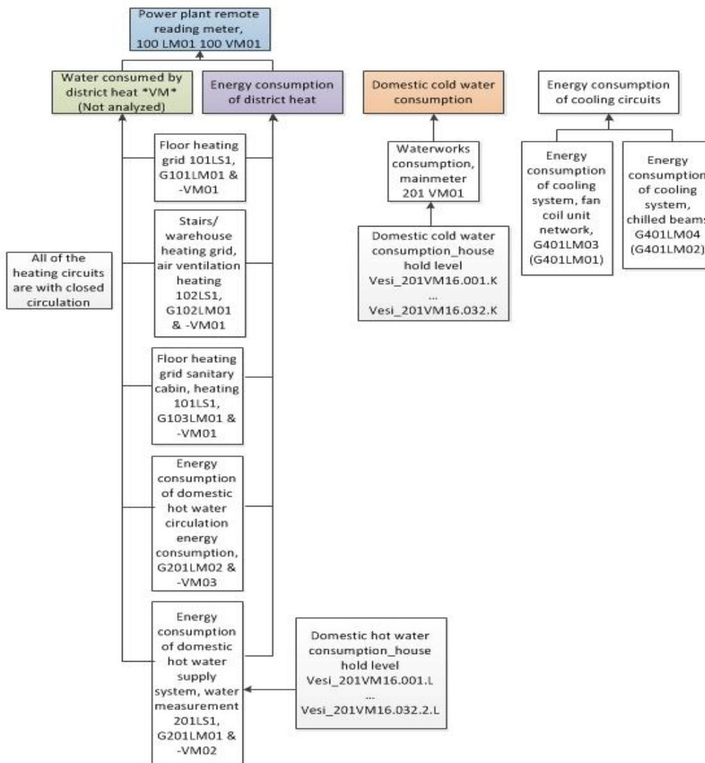
**Figure 27** Distributed heat, cool and hot water and cooling meters hierarchical structure
