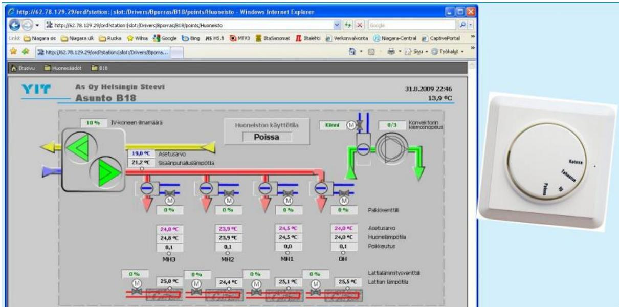
Figure 8 Monitoring interface top on Niagara framework
