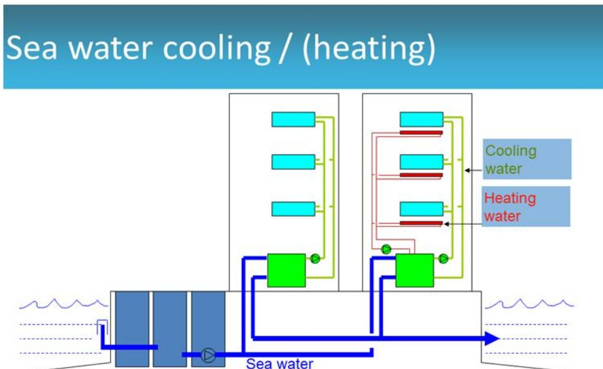
**Figure 5** Sea water cooling – (heating) chart
