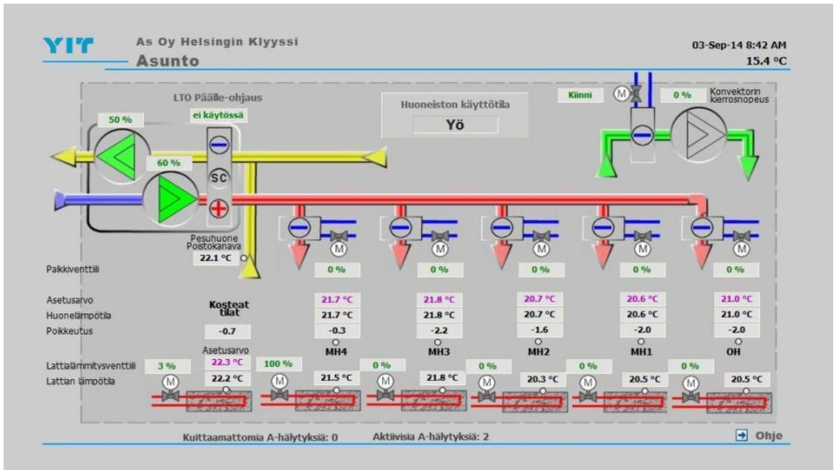
Figure 12 Apartment process view for remote controlling
