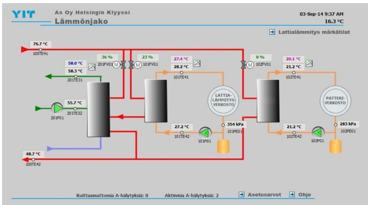
Figure 10 District heating process view for remote controlling
