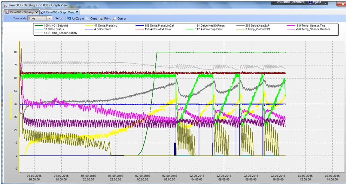
Figure 5: Graph showing the recorded values of temperatures, flows, pressure etc. for Test run 1.
