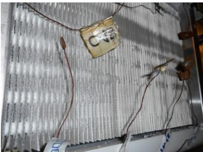
Figure 11: Finned surface – air inlet side
