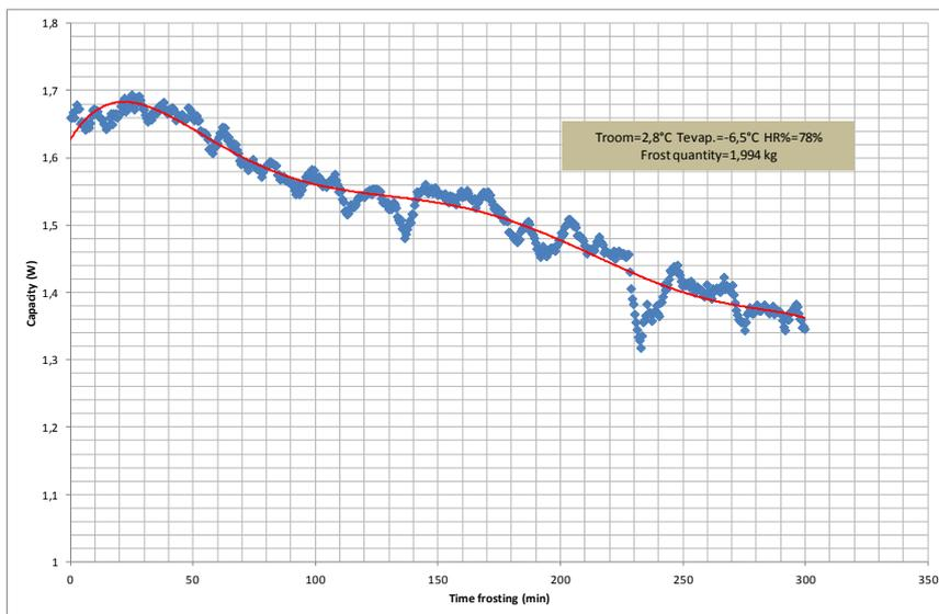
Figure 12: Cooling capacity – Frosting time (nano-structured surface)
