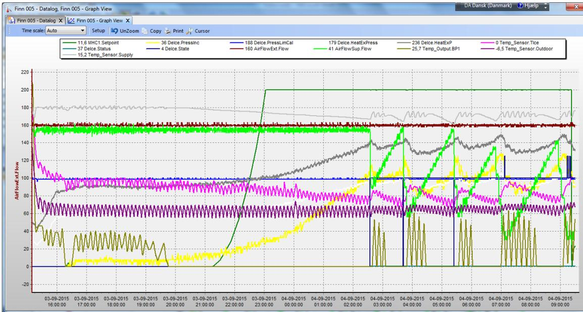
Figure 7: Graph showing the recorded values of temperatures, flows, pressure etc. for Test run 3.
