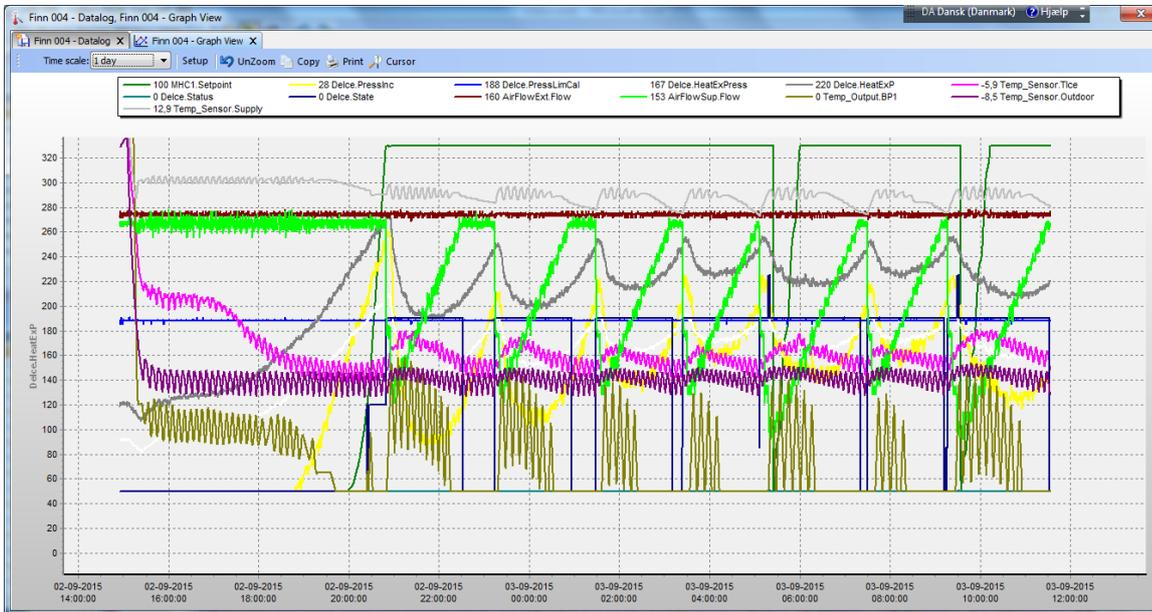
Figure 6: Graph showing the recorded values of temperatures, flows, pressure etc. for Test run 2.
