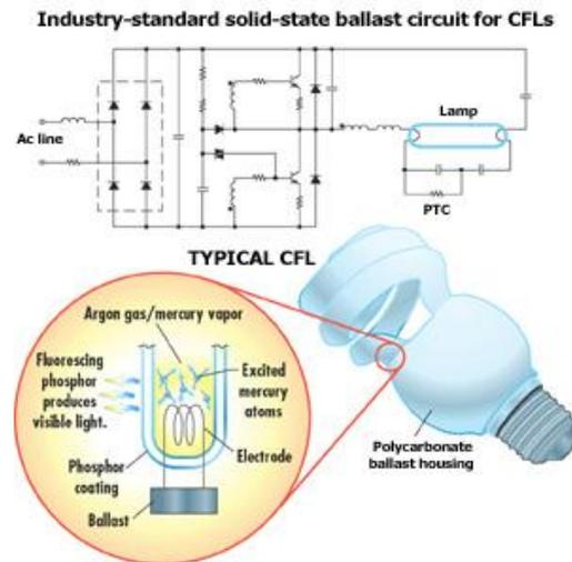
Figure 24 : Compact Lamps schematic representation
