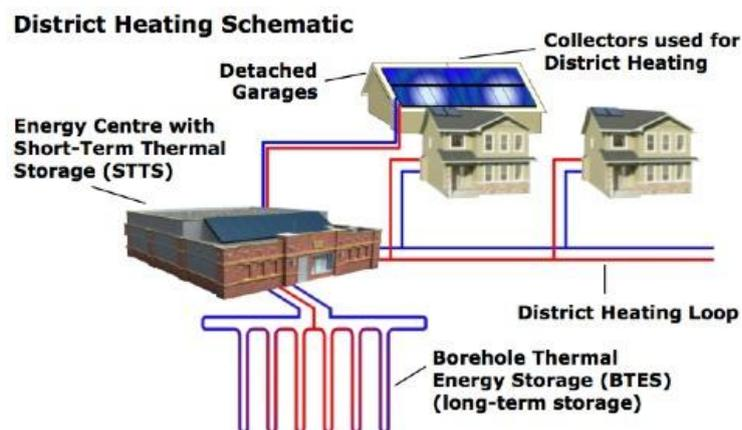
**Figure 42 : Schematic representation of a district heating installation**
