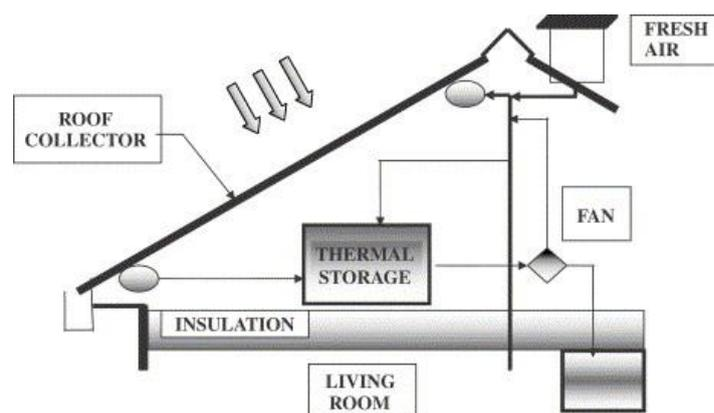
Figure 22: Solar heating system with PCM storage
