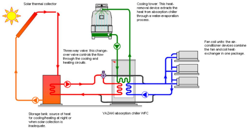
Figure 33 : Schematic representation of a solar absorption cooling system
