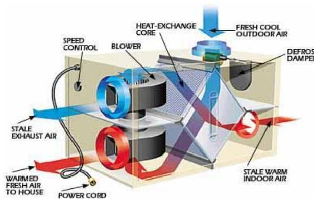
Figure 26 : Heat recovery ventilation system schematic
