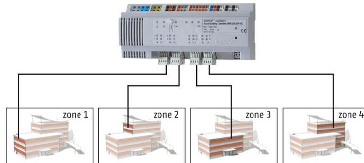
**Figure 30 : Schematic representation of a blind control system**
