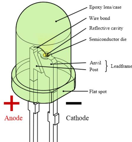
Figure 25 : LED schematic representation
