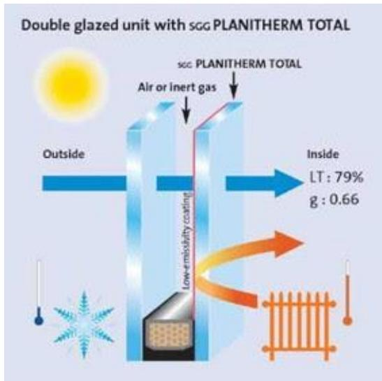
Figure 9 : Double glazing technology
