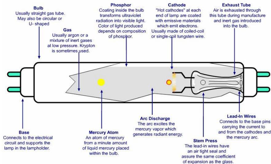
Figure 23 : Tubular lamps schematic representation
