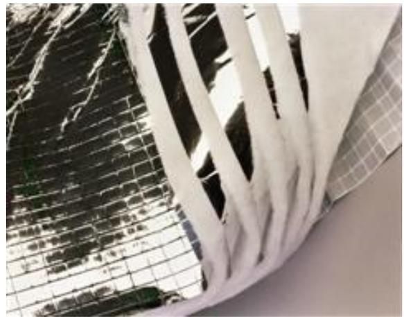
Figure 7 : Multi layers thermal insulation technology
