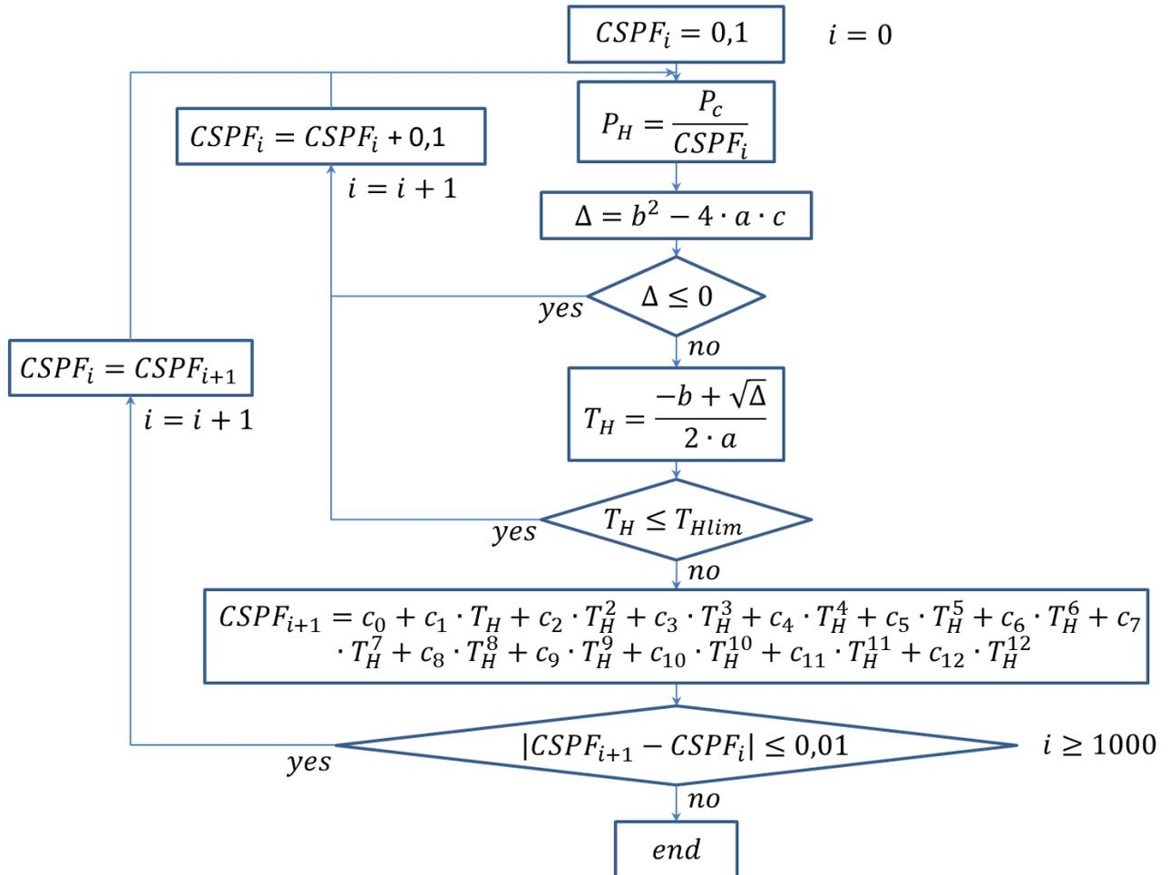
Figure 36: Algorithm used to compute the solar Absorption / Adsorption cooling CSPF
