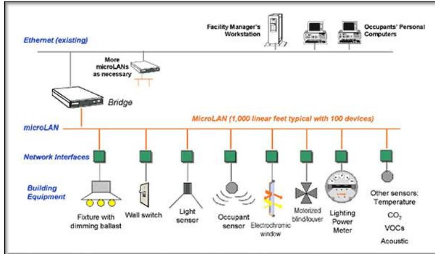
Figure 28 : Schematic representation of a lighting control system
