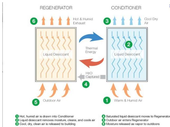
**Figure 32 : Schematic representation of a desiccant cooling system**
