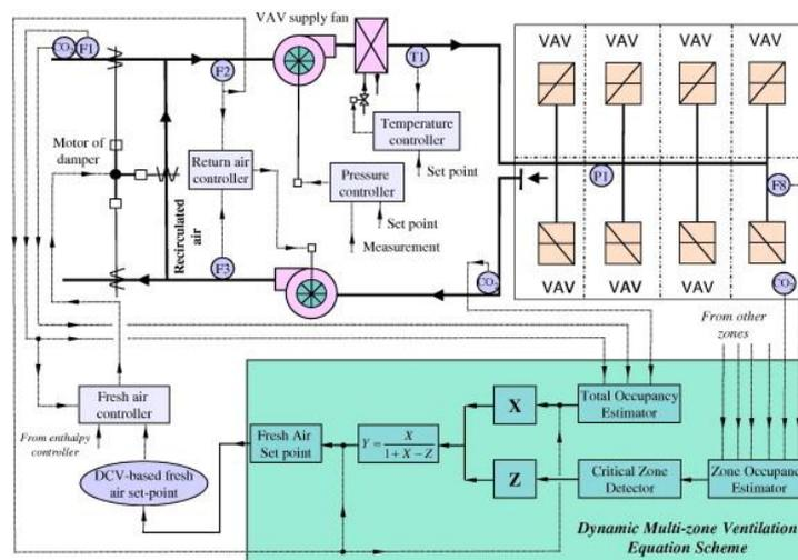
Figure 29: Schematic representation of a ventilation control system
