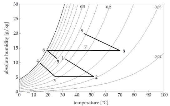
Figure 34 : Evaporative and desiccant cooling system description
