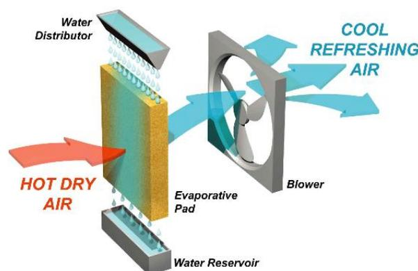
Figure 31 : Schematic representation of an evaporative cooling system
