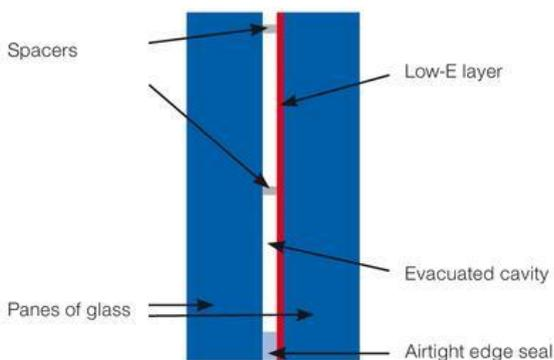
Figure 10 : Vacuum glazing technology
