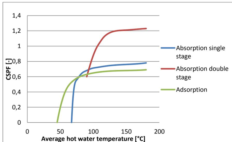
Figure 37: Performance of Absorption / Adsorption cooling systems – Influence of the average hot water temperature
