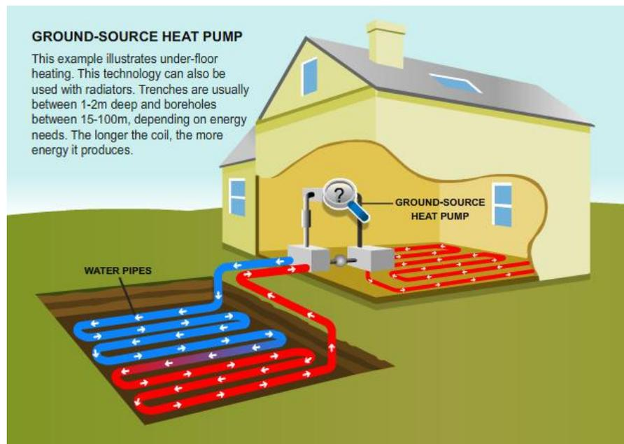
**Figure 40 : Ground source heat pump system**
