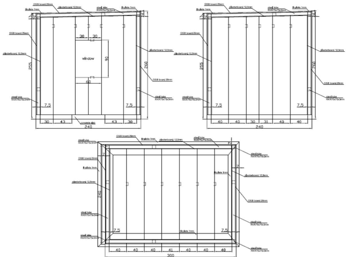
**Figure 27** Internal structure of the mock-ups
