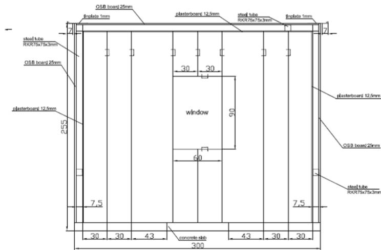
**Figure 26** Internal structure of the mock-ups
