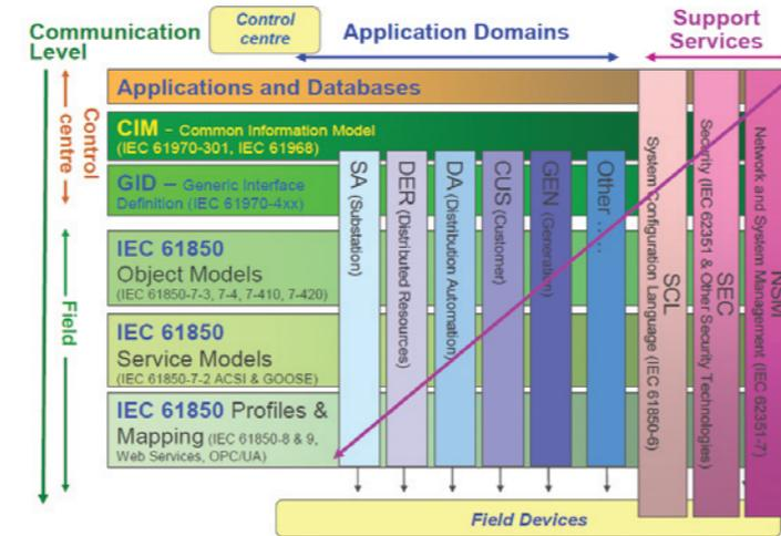
Figure 11: IEC 61850 models and the Common Information Model (CIM) [11]
