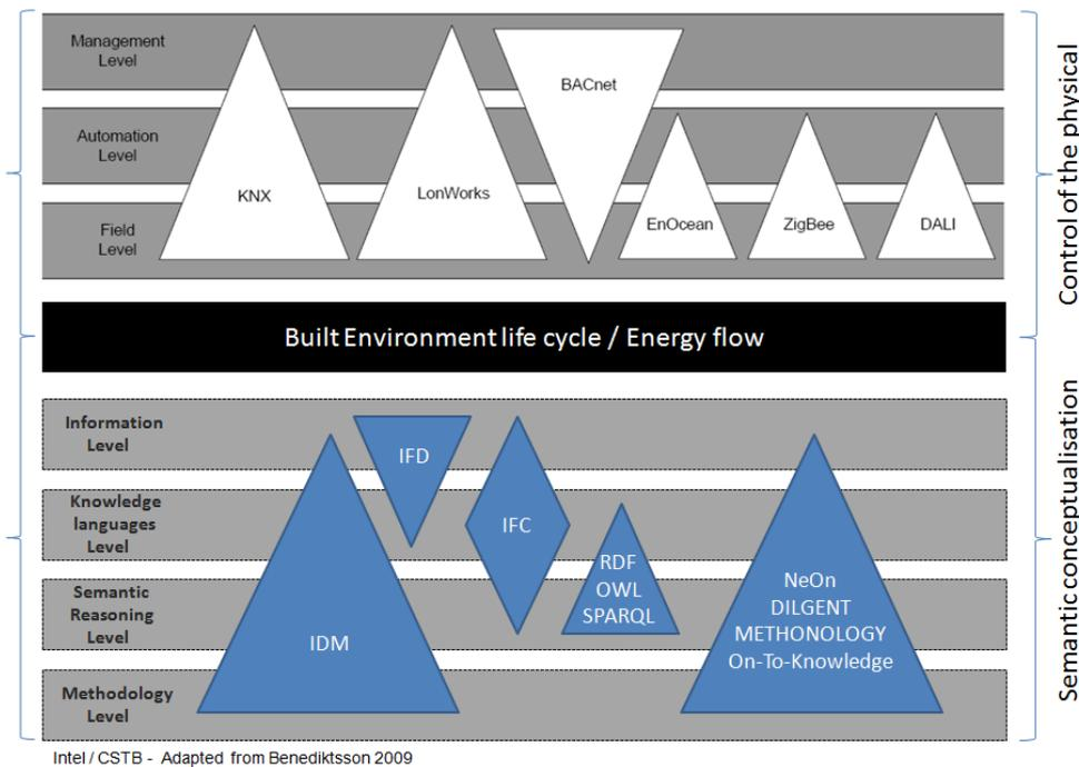
Figure 4: Mapping protocols / standards onto architectural levels of BMS / BAS
