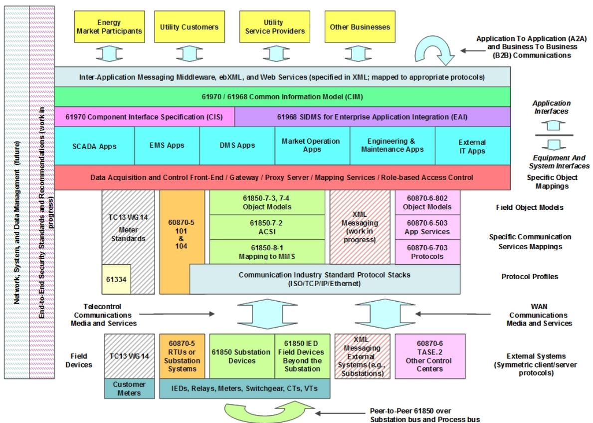
Figure 2: The IEC TC57 Reference Architecture
