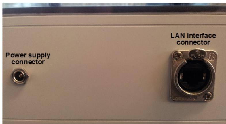
Figure 58: LAN interface and power supply connector of the APU
