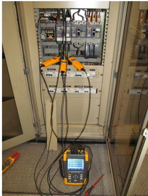
Figure 7. Analyser Fluke 435-II connected to one circuit of the station during the measurements.
