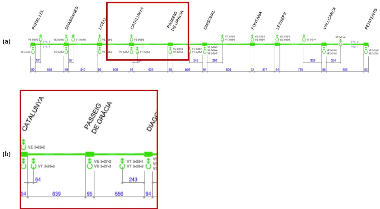
Figure 9. Location of fans along Line 3 in the segment stretching from PdG's station (a) and zoom centered on PdG-L3 (b).
