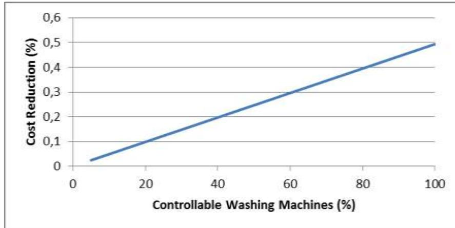
Figure 83 Consumer cost reduction as a function of controllable Washing Machines for price curve B
