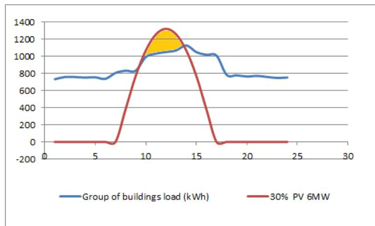
Figure 46 Energy curtailment for a group of buildings with PV installed capacity of 6MW
