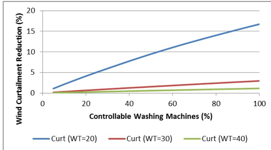
Figure 81 Wind curtailment reduction as a function of controllable Washing Machines for various levels of installed Wind capacity (MW)
