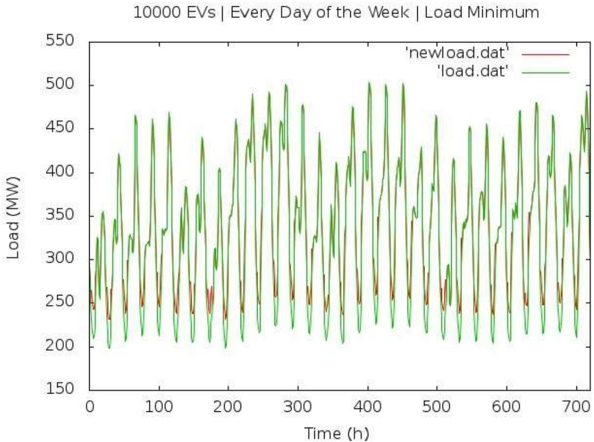
**Figure 88: 10000 Nissan Leaf Cars being charged every day of the week when the Load is minimal**
