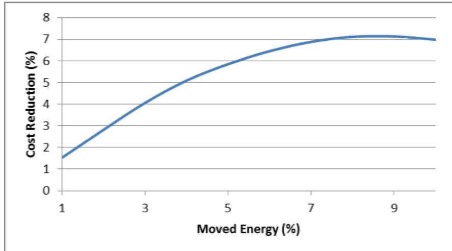
Figure 86 Cost reduction (%) as a function of the total energy moved (%) for 174 MW of installed wind power
