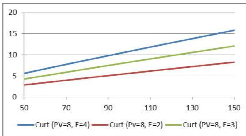
Figure 70 Curtailment reduction as a function of the number of washing machines for wash energy of 2-4kWh and installed PV capacity 8MW.
