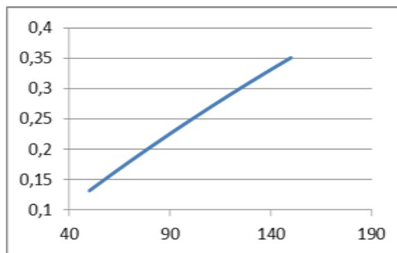
Figure 62 Cost reduction as a function of the number of HVAC devices for cost curve A
