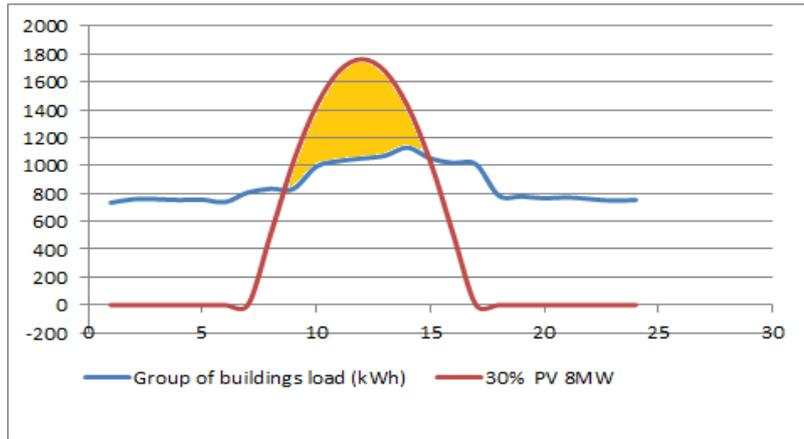
Figure 48 Energy curtailment for a group of buildings with PV installed capacity of 8MW.
