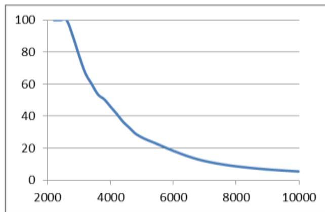
Figure 64 Curtailment reduction as a function of installed PV capacity for wash energy of 4kWh and 80 washing machines
