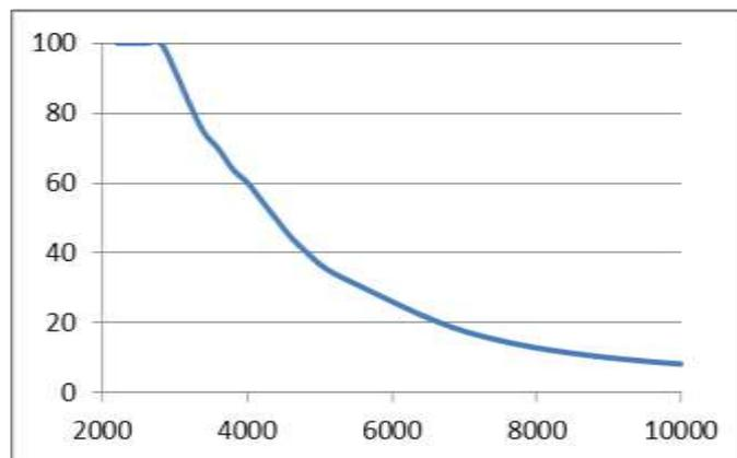
Figure 65 Curtailment reduction as a function of installed PV capacity for wash energy of 4kWh and 120 washing machines
