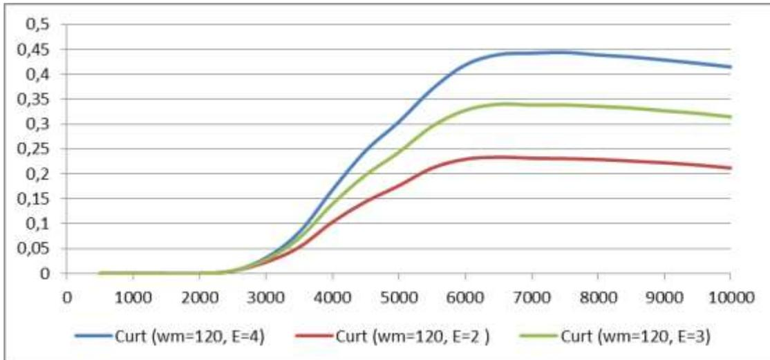
Figure 72 Reduction in PV investment payback time for feed-in tariff=0.25e/kWh and cost=0.1euros/kWh (120 washing machines)
