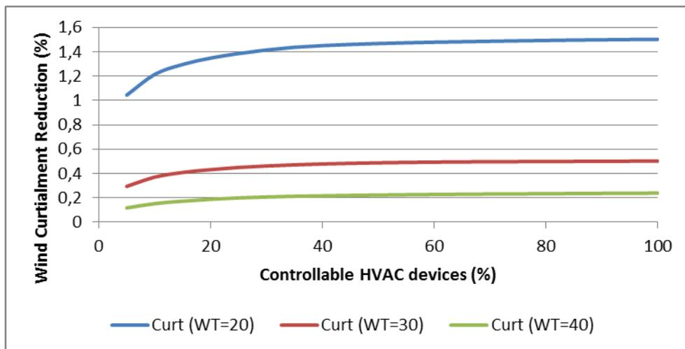
Figure 77 Wind curtailment reduction as a function of controllable HVAC for various levels of installed Wind capacity (MW)
