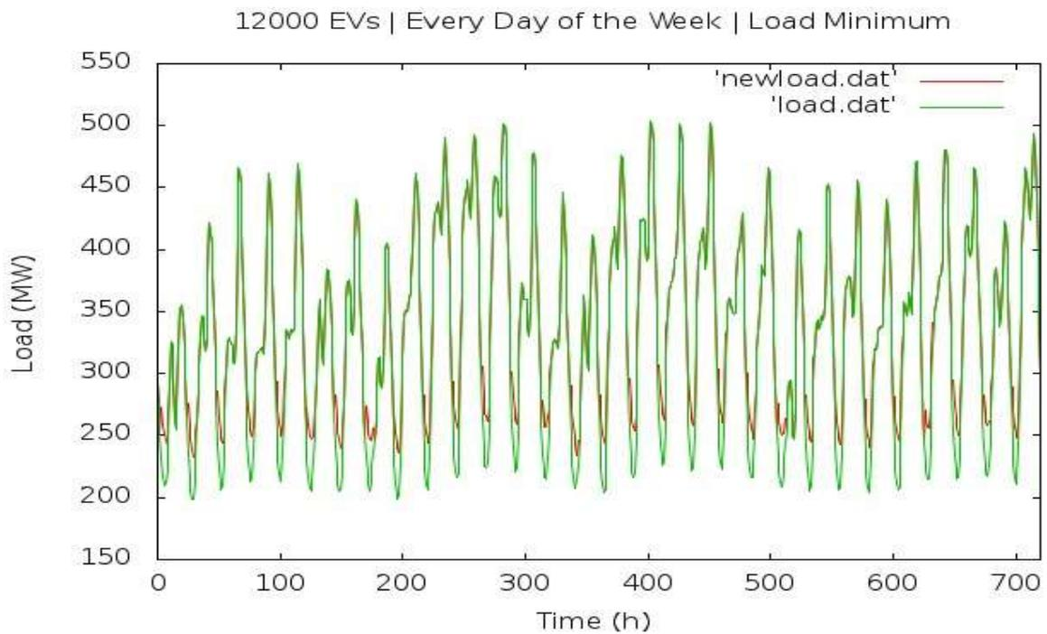
**Figure 90 12000 EVs being charged every day when the Load is Minimal**
