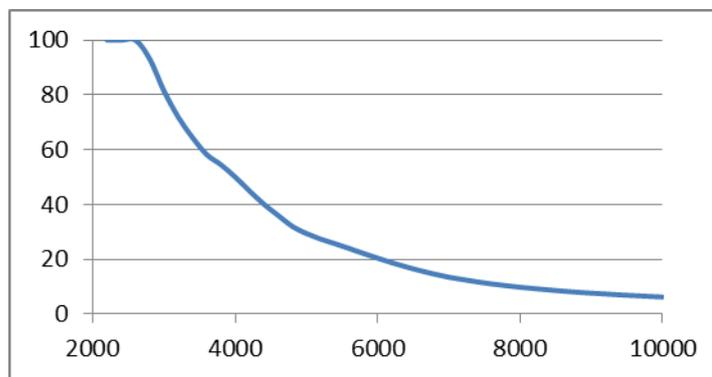
Figure 67 Curtailment reduction as a function of installed PV capacity for wash energy of 3kWh and 120 washing machines
