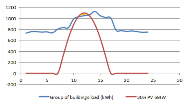
Figure 45 Energy curtailment for a group of buildings with PV installed capacity of 5MW.
