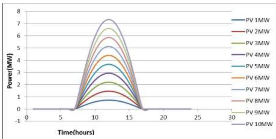
Figure 44 Typical PV production for 1-10MW photovoltaic generators.
