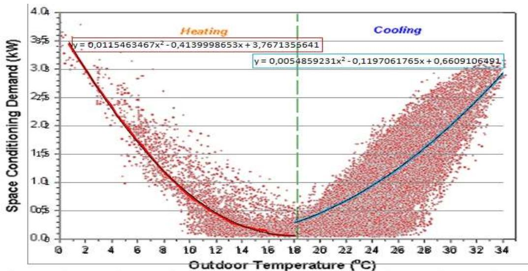
Figure 26 HVAC consumption curves
