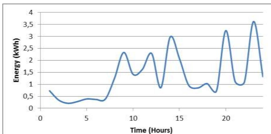
**Figure 24** Typical consumption of a small building (e.g. office, hospital etc) (for a day)
