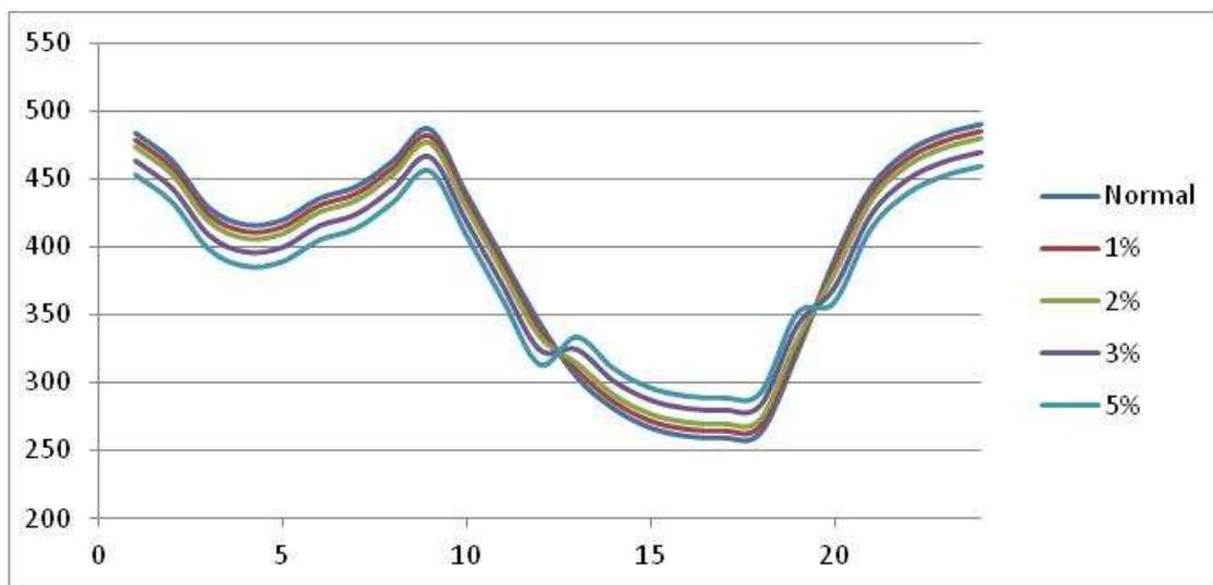
Figure 85 Load curves for the Island of Crete at 2012 for various levels of controllable load.
