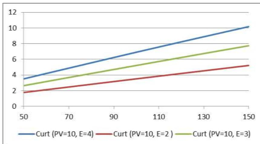
Figure 71 Curtailment reduction as a function of the number of washing machines for wash energy of 2-4kWh and installed PV capacity 10 MW.
