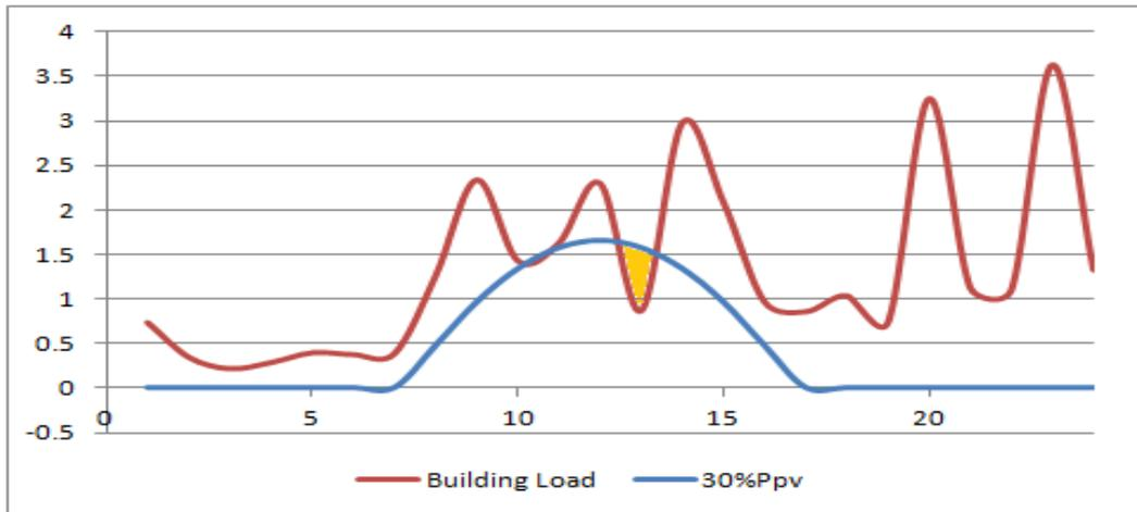
Figure 27 Energy curtailment for a building with PV installed capacity of 10kW.
