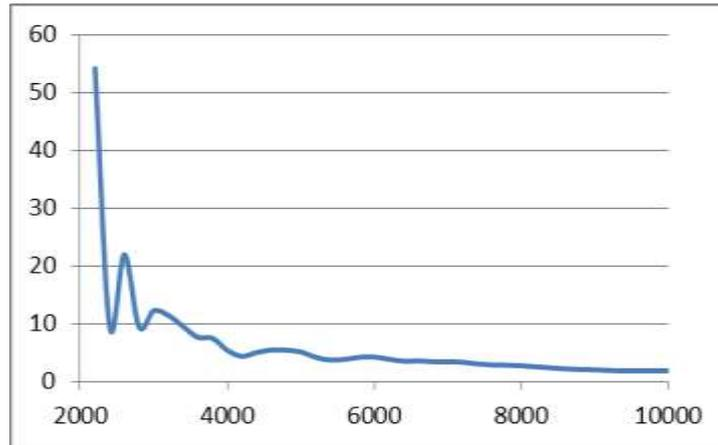
Figure 58 PV curtailment reduction as a function of the installed PV capacity 100 HVAC devices and hot year/place
