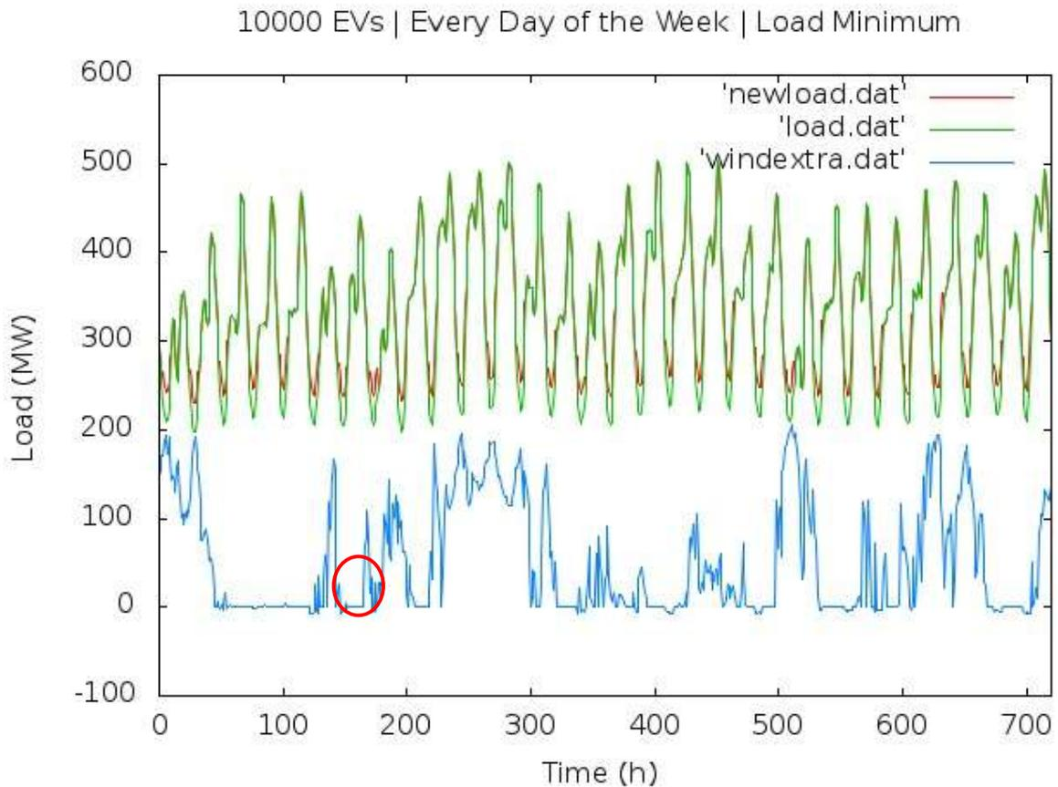
**Figure 89: 10000 Leaf Cars charging every day at minimal load times plus wind power penetration**
