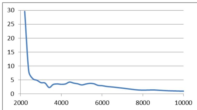
Figure 59 PV curtailment reduction as a function of the installed PV capacity 50 HVAC devices and cold year
