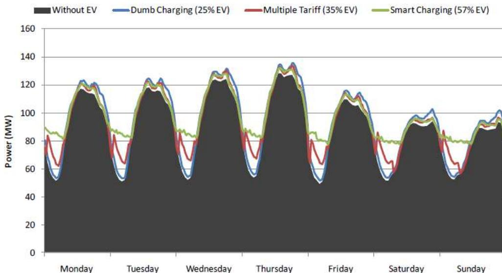
**Figure 10** Load profiles without and with EV (MV Network 1)
