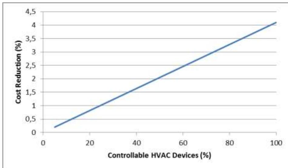
Figure 79 Consumer cost reduction as a function of controllable HVAC for price curve B
