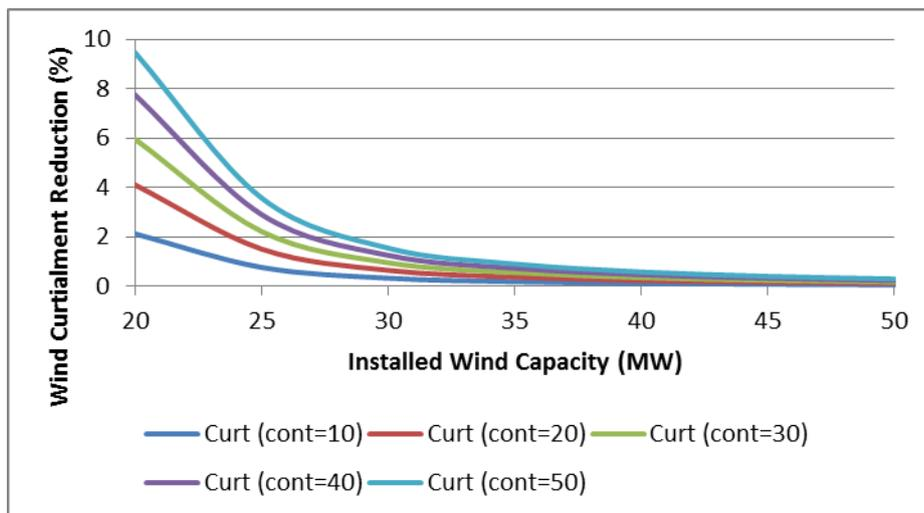
**Figure 80 Wind curtailment reduction as a function of the installed Wind capacity (MW) for various levels of controllable Washing Machines**
