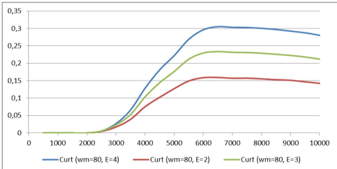
Figure 73 Reduction in PV investment payback time for feed-in tariff=0.25e/kWh and cost=0.1euros/kWh (80 washing machines)
