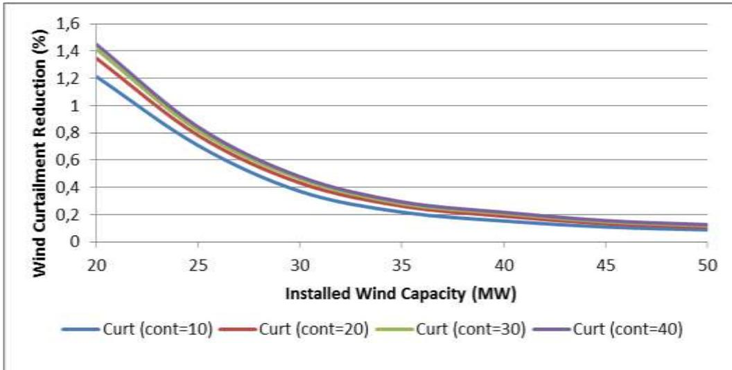
Figure 76 Wind curtailment reduction as a function of the installed Wind capacity (MW) for various levels of controllable HVAC
