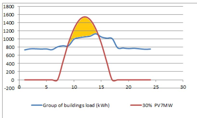
Figure 47 Energy curtailment for a group of buildings with PV installed capacity of 7MW.
