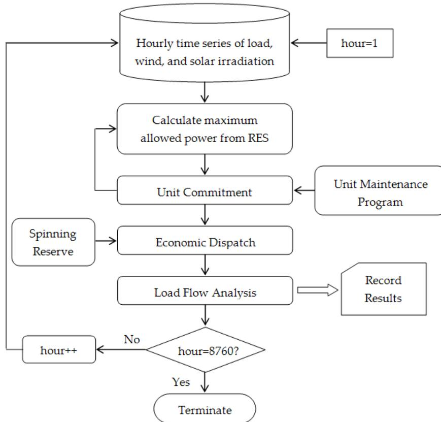
Figure 84 Hourly simulation flowchart for the steady-state analysis
