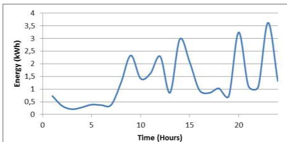
Figure 14 load curve of a small building
