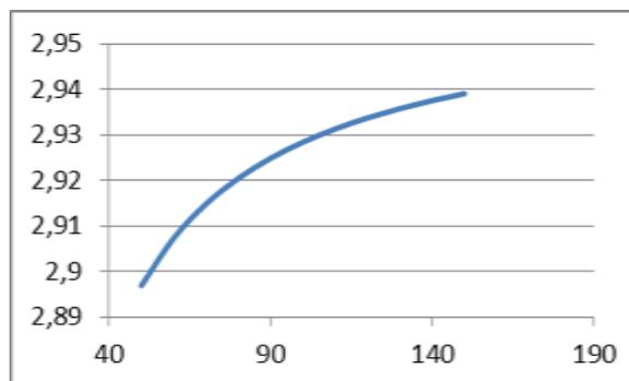
Figure 63 Cost reduction as a function of the number of HVAC devices for cost curve B
