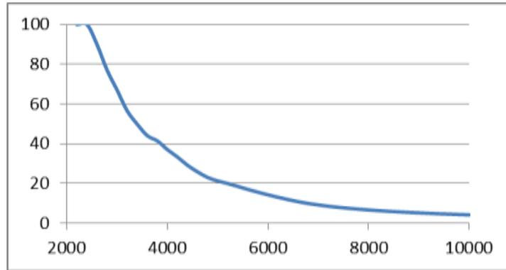
Figure 66 Curtailment reduction as a function of installed PV capacity for wash energy of 3kWh and 80 washing machines
