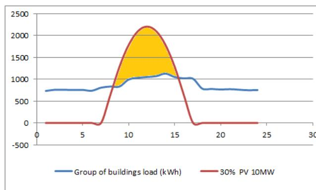
Figure 50 Energy curtailment for a group of buildings with PV installed capacity of 10MW.
