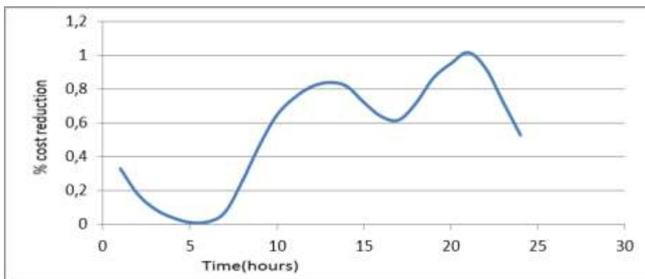
Figure 41 Cost reduction as a function of the time of wash for cost curve B and wash energy of 0.5kWh
