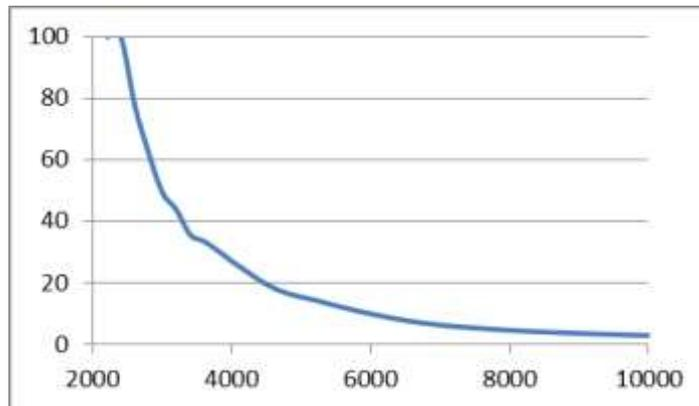
Figure 68 Curtailment reduction as a function of installed PV capacity for wash energy of 2kWh and 80 washing machines
