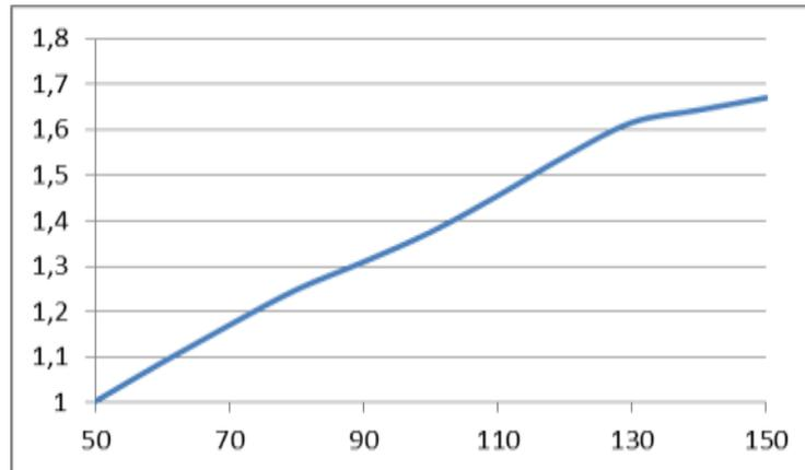
**Figure 56 PV curtailment reduction as a function of the number of HVAC devices for installed PV capacity of 10 MW**
