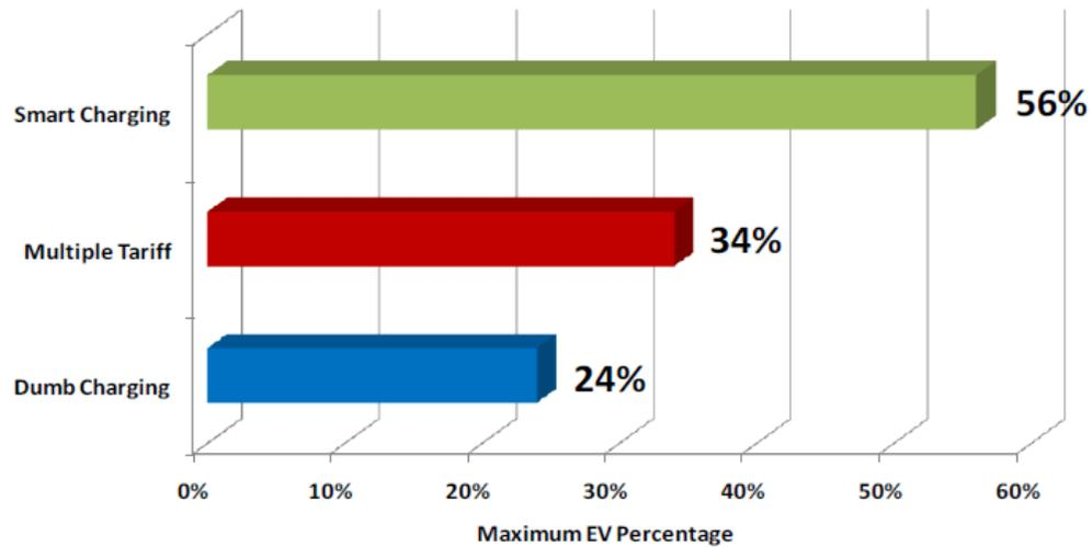
**Figure 7** Maximum EV integration percentage in the MV Network 1
