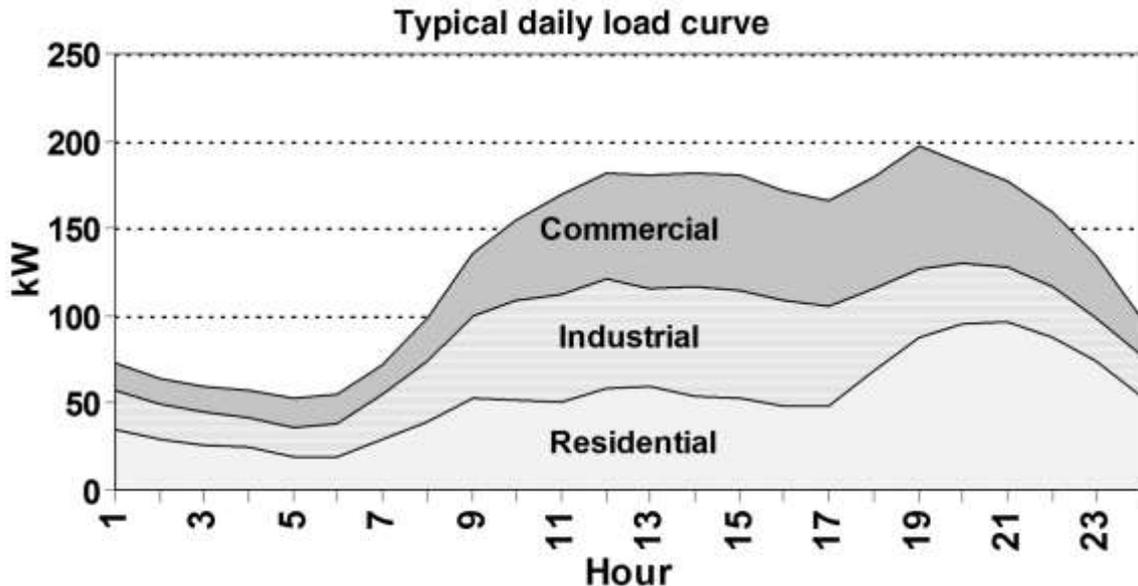
**Figure 5 Typical load curve for each feeder of the study case network**
