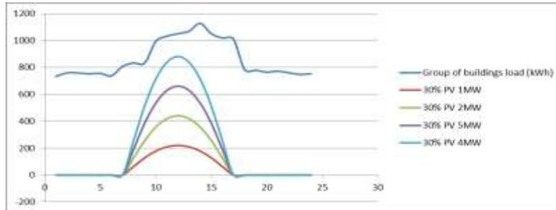
Figure 51 there is no energy curtailment for a group of buildings with PV installed capacity of 1-4MW.
