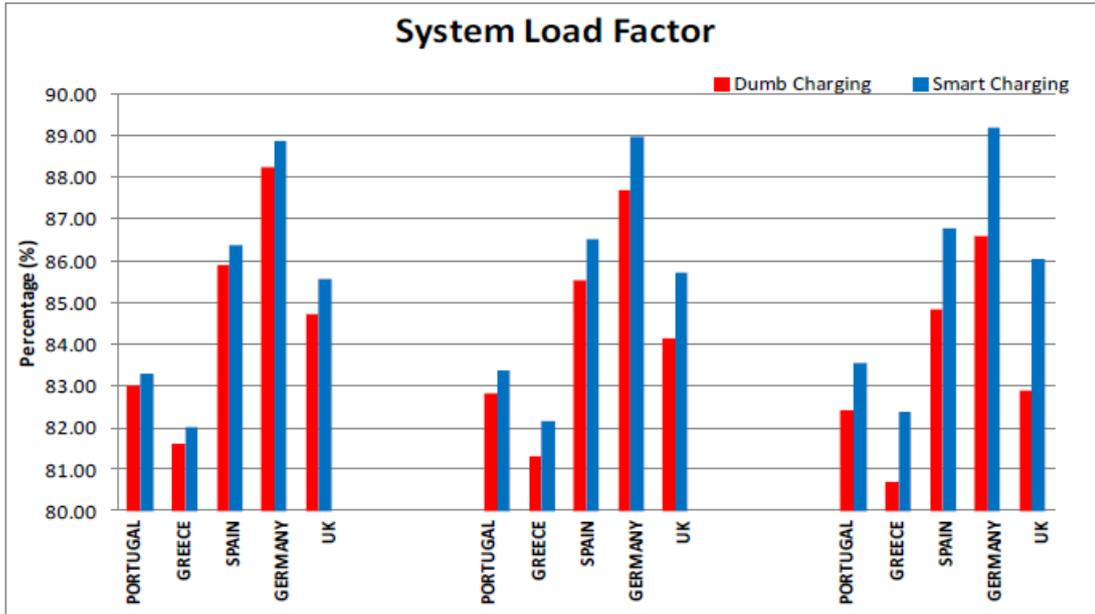
**Figure 9** The increase of system load factor comparing “dumb charging” with “smart charging” (Home charging- winter)
