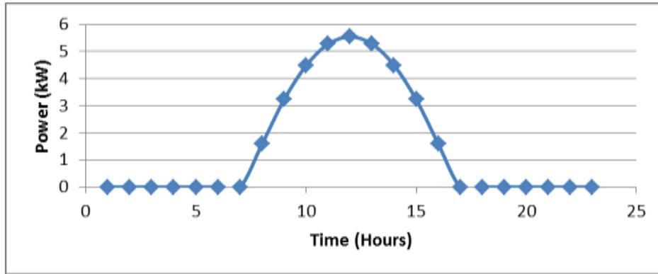
Figure 25 Typical PV production for a 10kW photovoltaic generator
