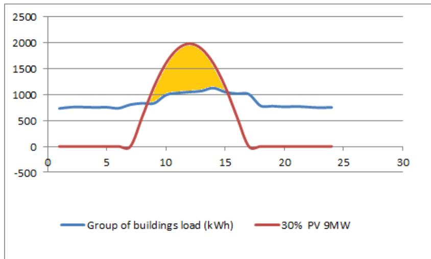
Figure 49 Energy curtailment for a group of buildings with PV installed capacity of 9MW
