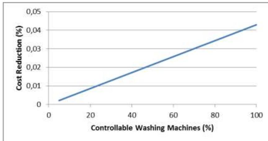
Figure 82 Consumer cost reduction as a function of controllable Washing Machines for price curve A
