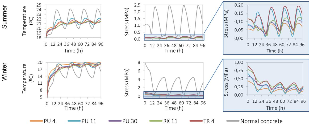
Figure 13: Temperature on the interior of the wall and von Mises stresses in its center, for summer and winter conditions, for walls made of blocks (20 cm thick) composed by different concrete mixtures, including normal concrete
