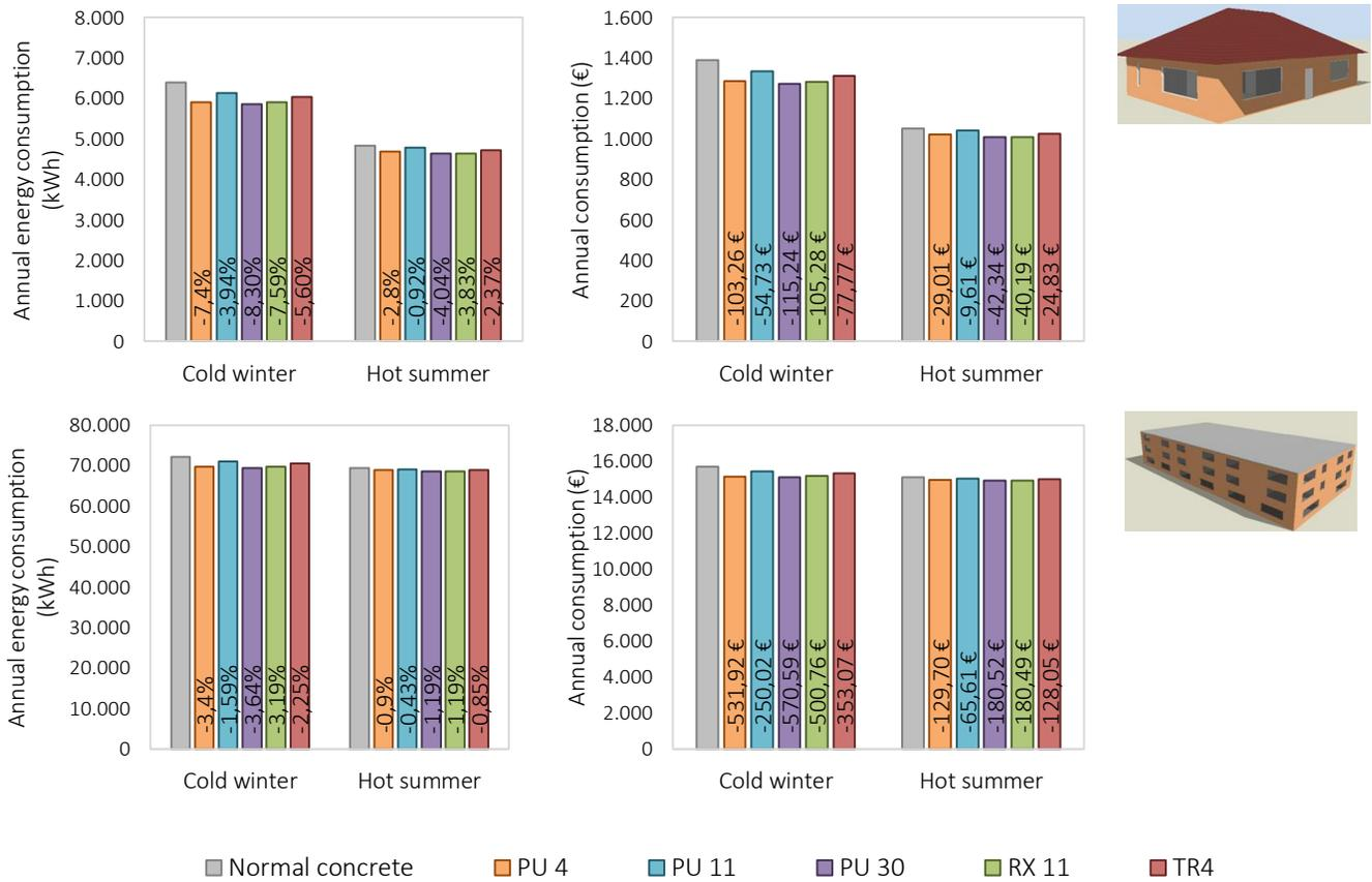
Figure 17: Energy consumption and corresponding costs for façade walls made of blocks, for summer and winter, and for one-story and multi-story buildings
