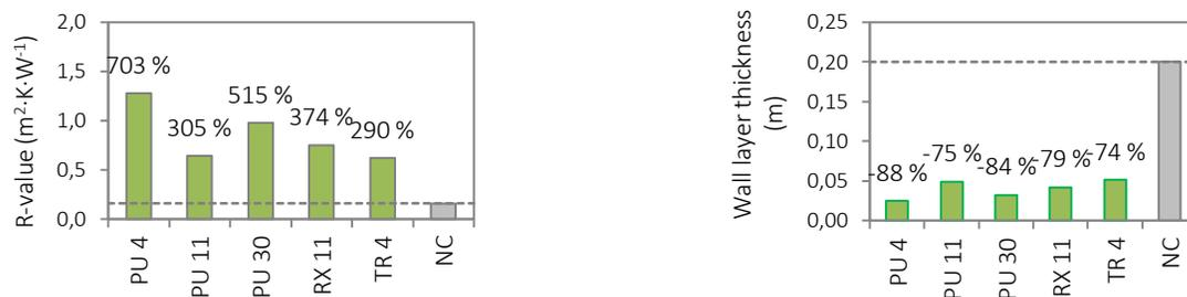
Figure 8: Thermal insulation (R-value) of a wall made of blocks (0.20 m thick) composed by different concrete mixtures, including normal concrete, and thickness of a wall made of different concrete mixtures, that results in the same thermal insulation of a wall made of normal concrete with 0.20 m thickness
