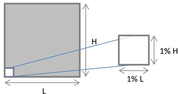
Figure 7. Area of the domain considered for calculating the maximum stress (grey) and portion of the domain excluded (white) equivalent to 0.01% of all domain
