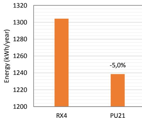
Figure 22. Energy necessary to keep temperature between 18°C and 25 °C in the mock-up interior, when walls are composed by RX4 and PU21 panels
