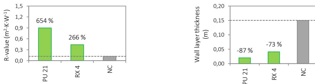
Figure 9: Thermal insulation (R-value) of a wall made of panels (0.15 m thick) composed by different concrete mixtures, including normal concrete, and thickness of a wall made of different concrete mixtures, that results in the same thermal insulation of a wall made of normal concrete with 0.15 m thickness
