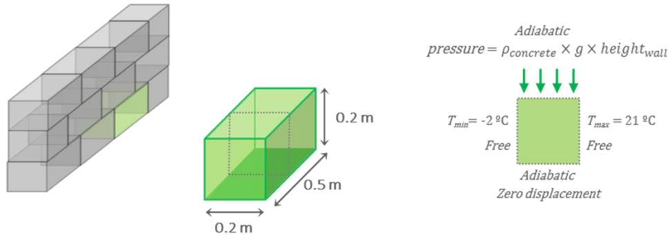
Figure 1: Dimensions and boundary conditions considered for analyzing the thermal and mechanical behavior of a concrete block
