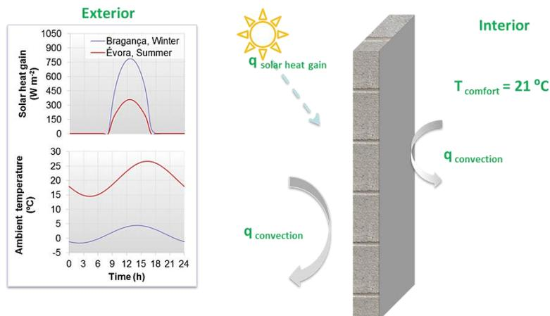
Figure 12: Façade wall and climatic conditions considered
