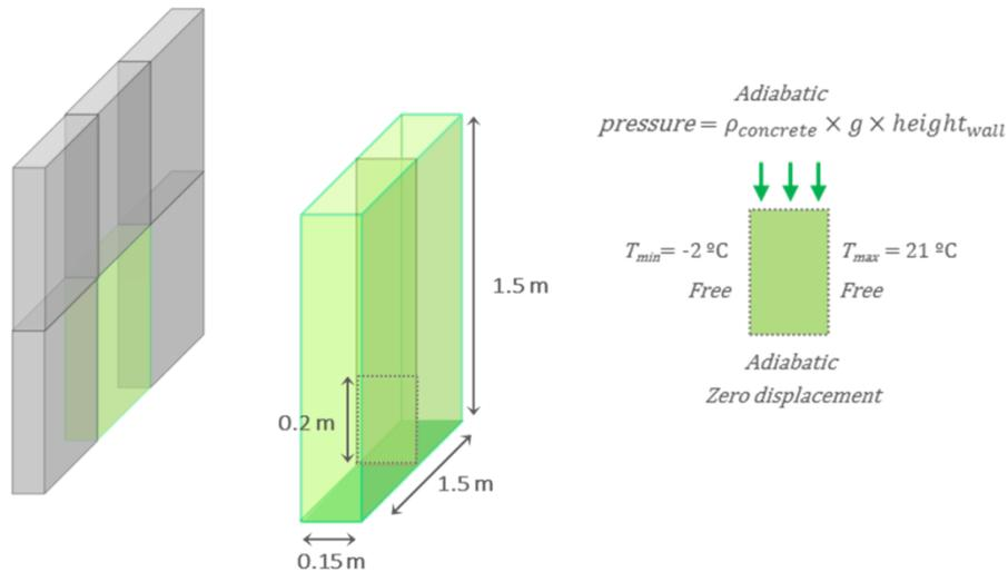
Figure 2: Dimensions and boundary conditions considered for analyzing the thermal and mechanical behavior of a concrete panel
