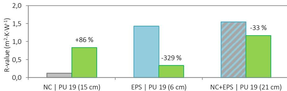
Figure 10. Thermal insulation provided by: one layer of NC (15 cm thick) and of PU 19 (15 cm thick); one layer of EPS (6 cm thick) and of PU 19 (6 cm thick); a multilayer composed by NC (15 cm thick) and EPS (6 cm thick) and one layer of PU 19 (21 cm thick)
