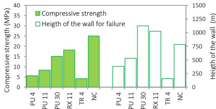
Figure 5: Compressive strength and height of the wall made of blocks to promote failure, for each concrete mixture, considering thermal expansion phenomena
