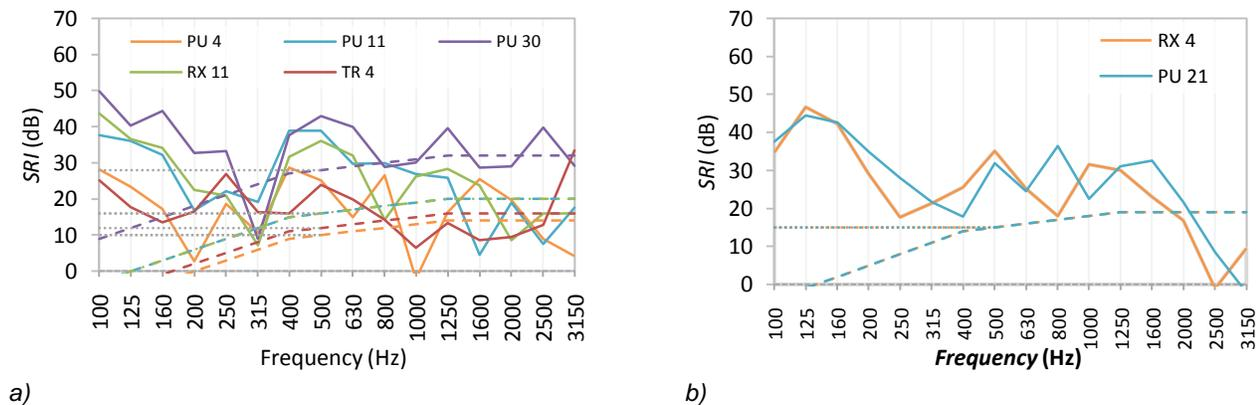
Figure 15. Sound reduction index (solid lines) obtained for walls made of: a) blocks composed by corresponding mixtures and b) panels composed by corresponding mixtures; shifted reference curve (dashed-lines) and weighted sound reduction index (dotted-line) are shown for each mixture
