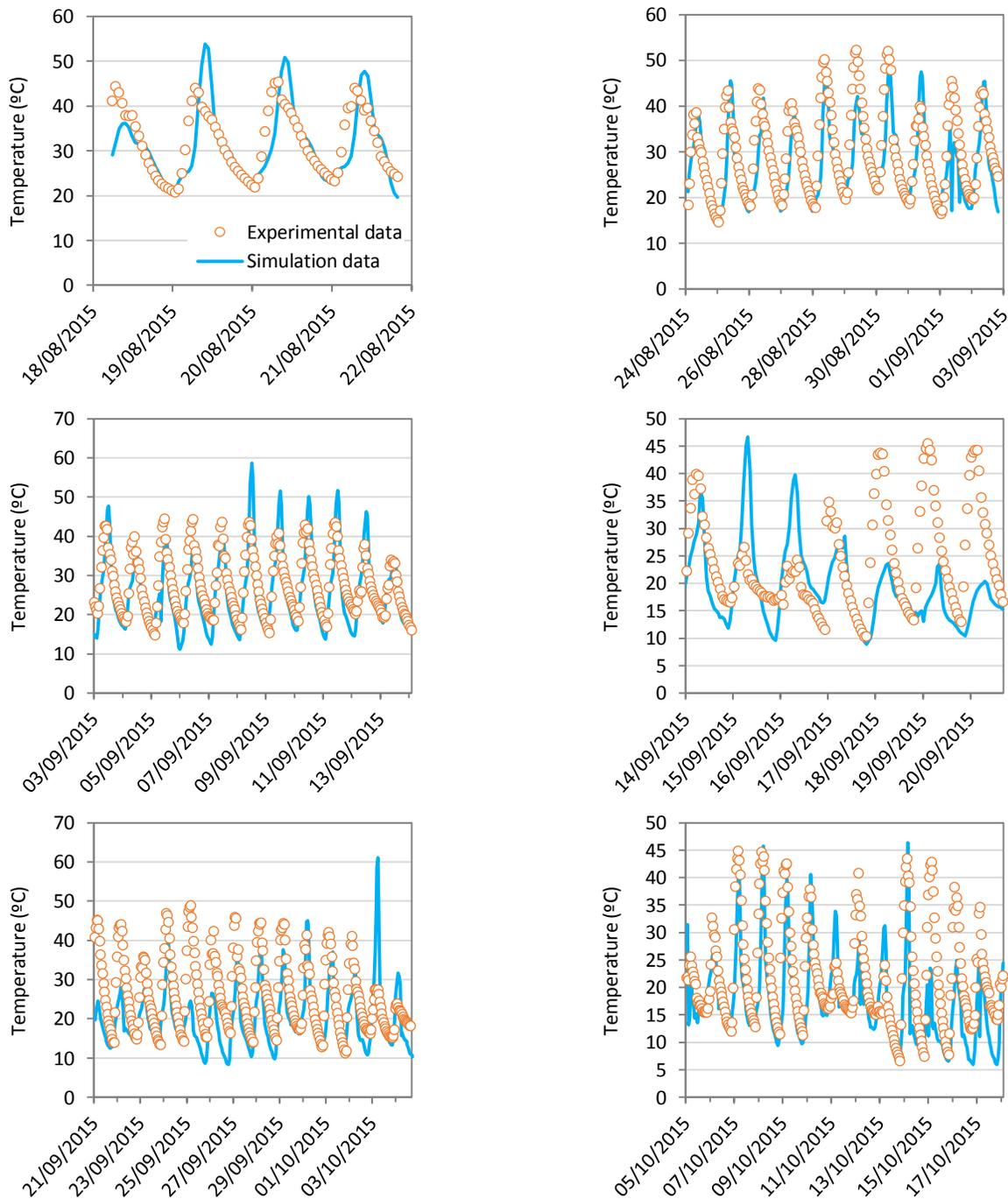
Figure 21. Temperature in the west wall of the mock-up made of RX4 panels: experimental and simulated data
