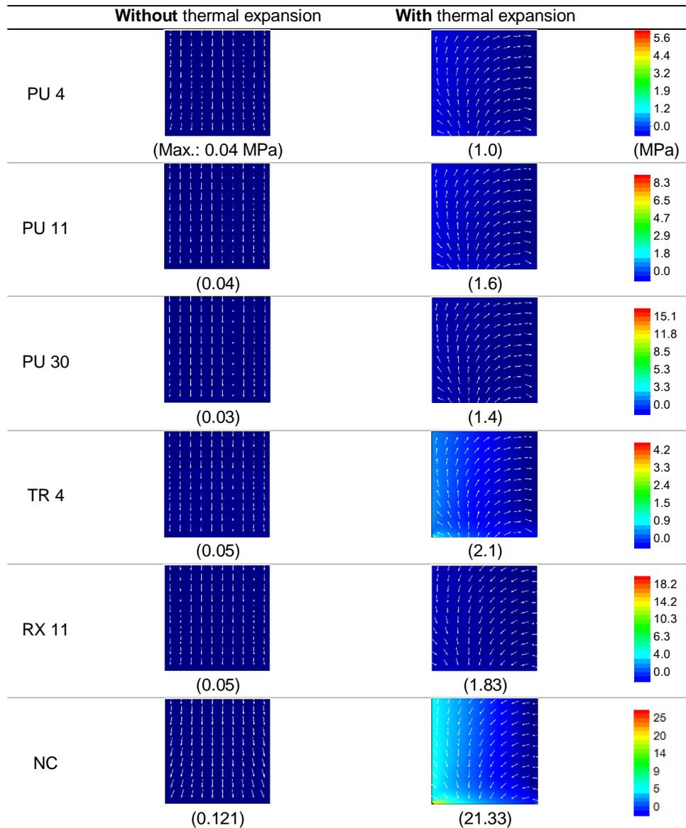
Figure 3: von Mises stress distribution (MPa), with and without thermal expansion phenomena, and arrows showing the direction of the deformation, for blocks; maximum stress obtained is reported
