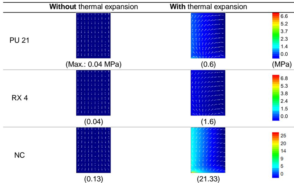
Figure 4: von Mises stress distribution (MPa), with and without thermal expansion phenomena, and arrows showing the direction of the deformation when thermal expansion is considered, for panels; maximum stress obtained is reported
