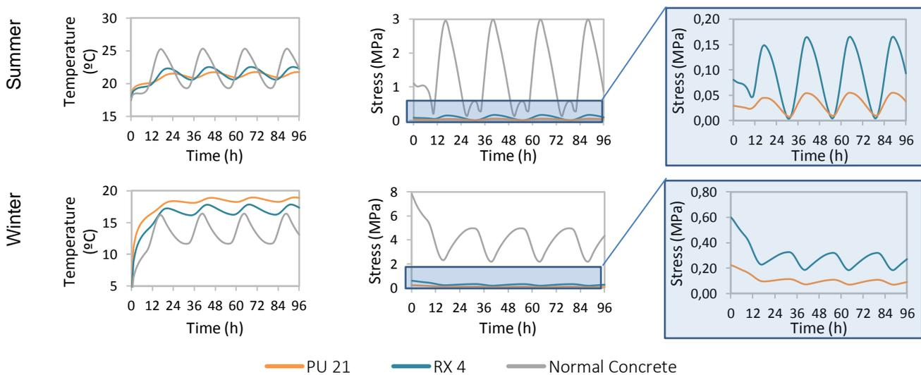
Figure 14: Temperature on the interior of the wall and von Mises stresses in its center, for summer and winter conditions, for walls made of panels (15 cm thick) composed by different concrete mixtures, including normal concrete
