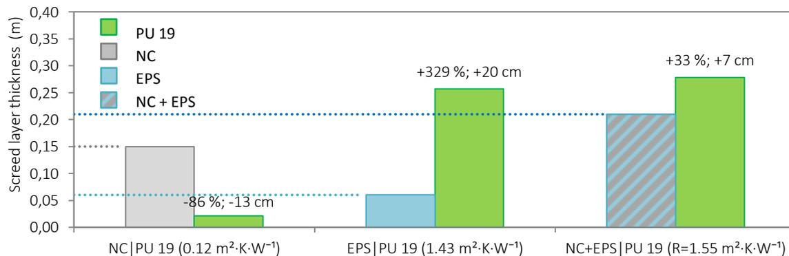
Figure 11. Thickness of PU 19 layer that provides the same thermal insulation of: one layer of NC (15 cm thick), one layer of EPS (15 cm thick) and a multilayer composed by 15 cm of NC and 6 cm of EPS
