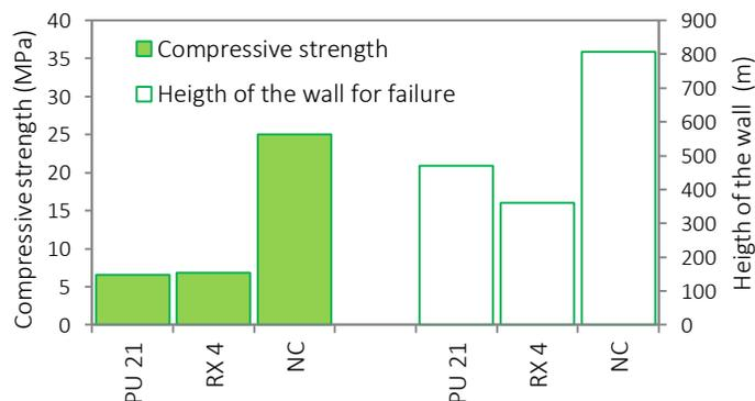
Figure 6: Compressive strength and height of the wall made of panels to promote failure, for each concrete mixture, considering thermal expansion phenomena
