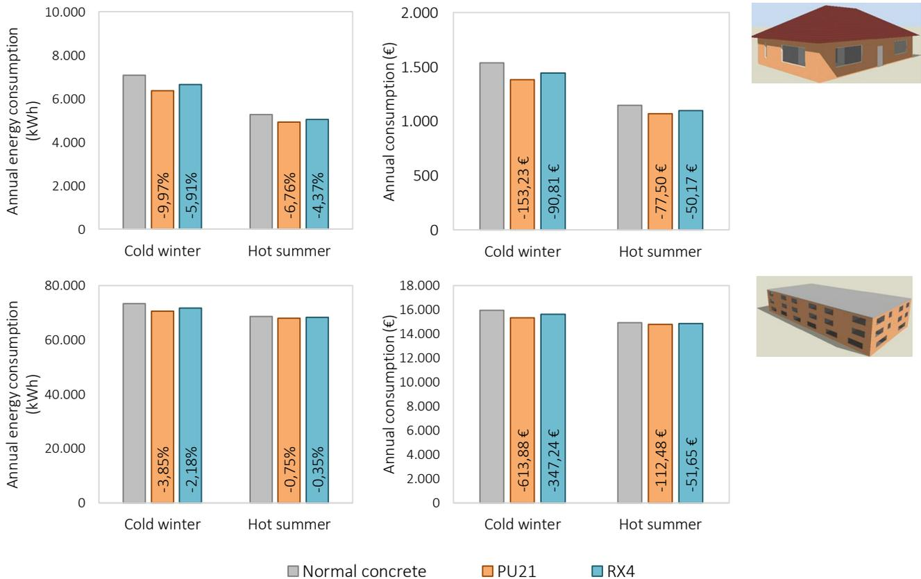
Figure 18: Energy consumption and corresponding costs for façade walls made of panels, for summer and winter, and for one-story and multi-story buildings
