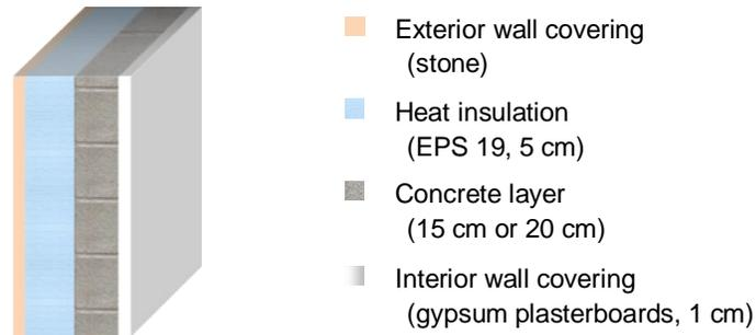
Figure 16. Schematics of a simple multilayer façade wall configuration
