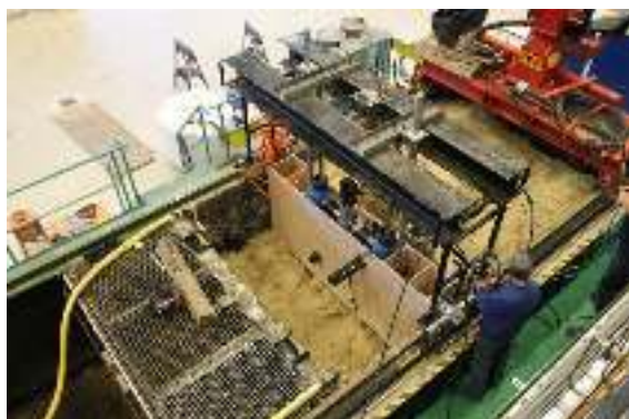
Deltares GeoModel container (4 x 2.5 x 1.2 m)
