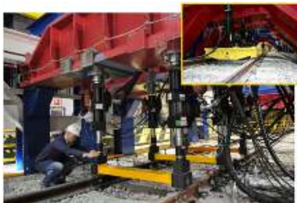
CEDEX railway track simulator (21 x 5 x 4 m)
